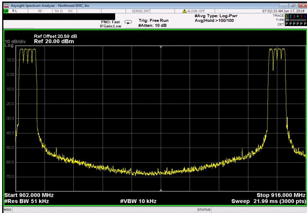
Hopping Mode, Spreading Factor 10, Upper and Lower Channel Sets
