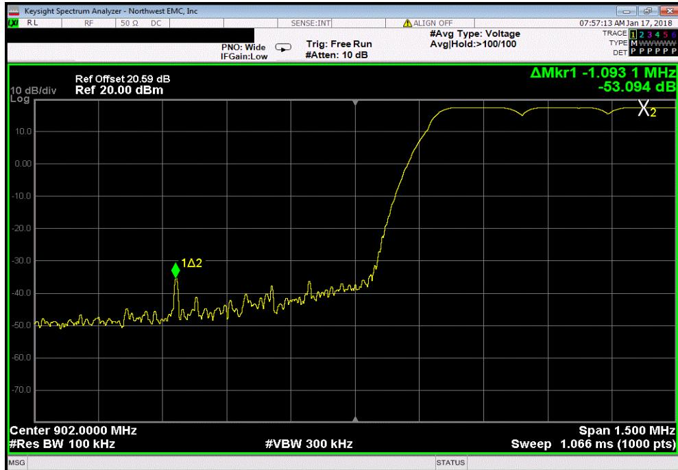
Hopping Mode, Spreading Factor 7, Upper Band Edge, 928 MHz
