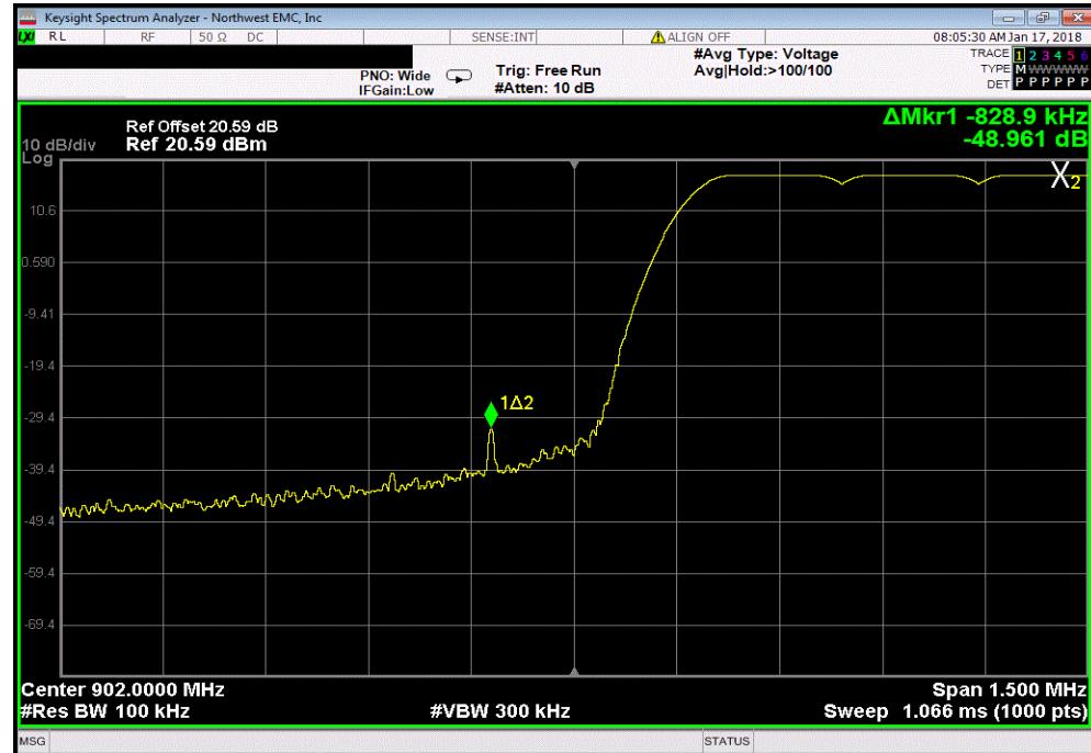
Hopping Mode, Spreading Factor 10, Upper Band Edge, 928 MHz
