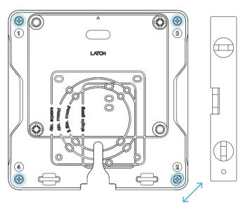
Install Mounting Plate. Attach to junction box or attach to wall or ceiling.
