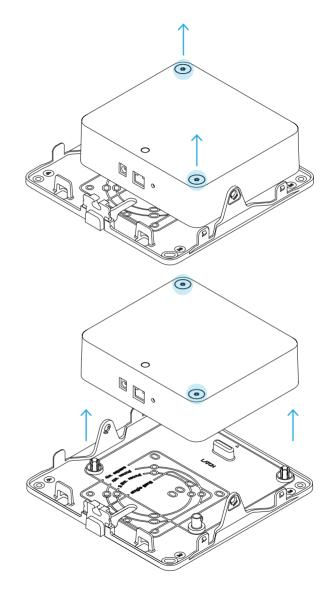
Rotate Torx screws in Hub counter-clockwise to unlock. Remove the Hub from the Mounting Plate.
