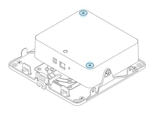
Attach Hub to Mounting Plate by aligning mating features.
