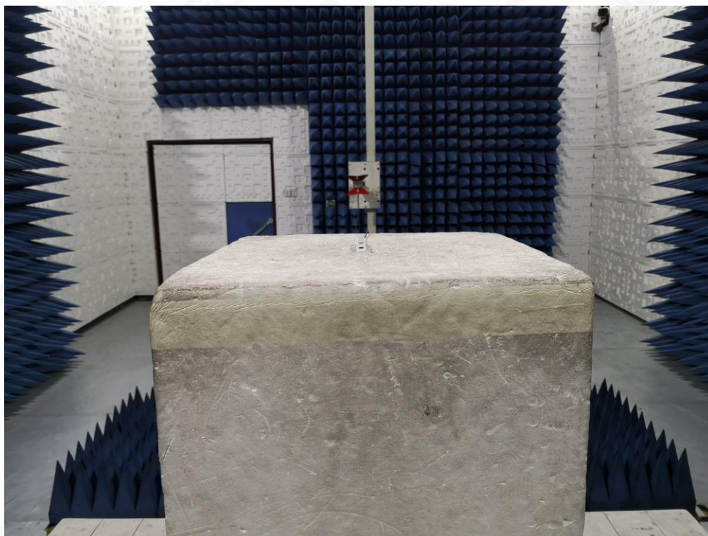
RADIATED EMISSION TEST SETUP ABOVE 1GHZ
