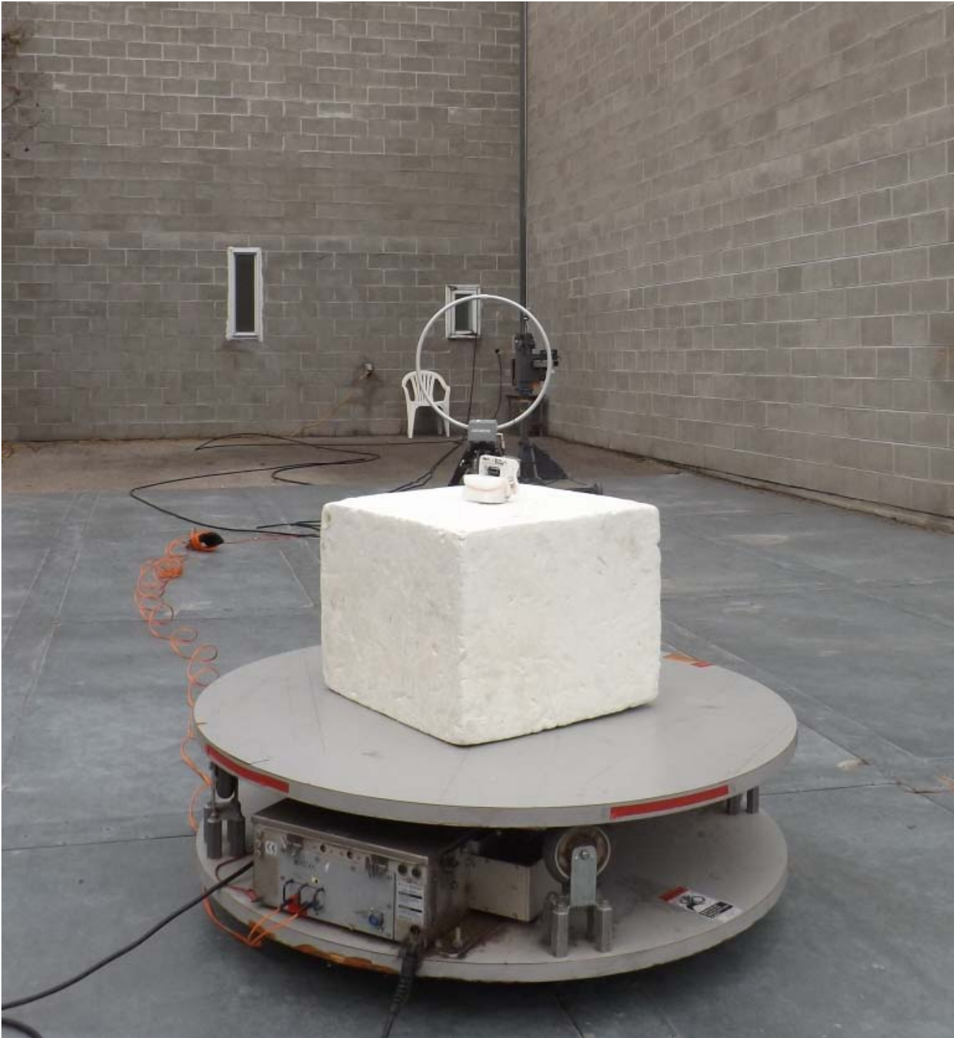
Figure E23.2 – Setup, Radiated Emissions Measurements Below 30MHz
