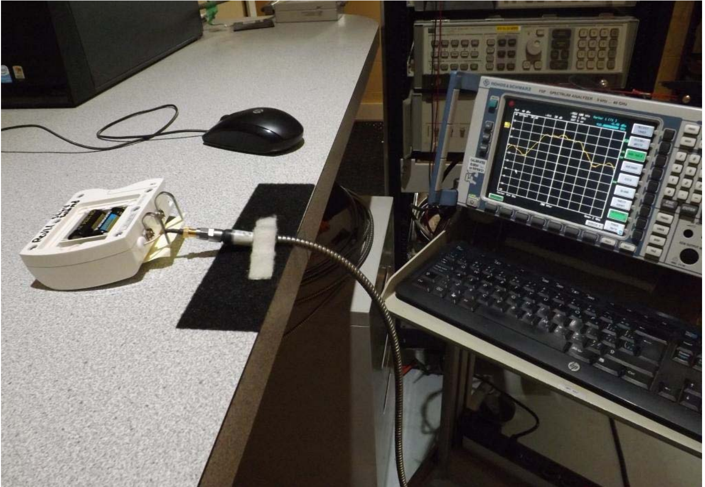
Figure E23.1 – Setup, Antenna Port Conducted Measurements
