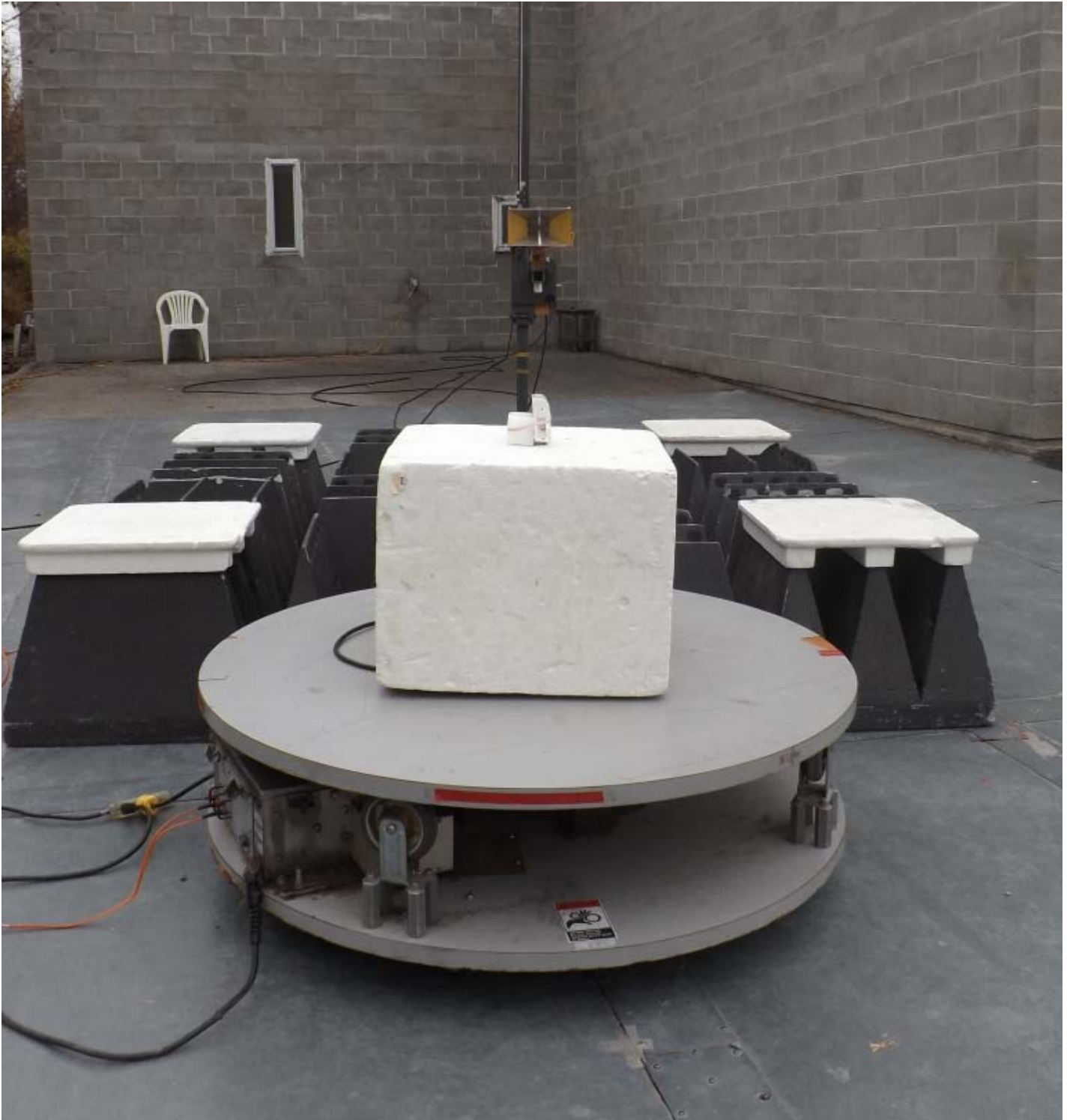
Figure E23.5 – Setup, Radiated Rx Emissions Measurements Above 1000MHz
