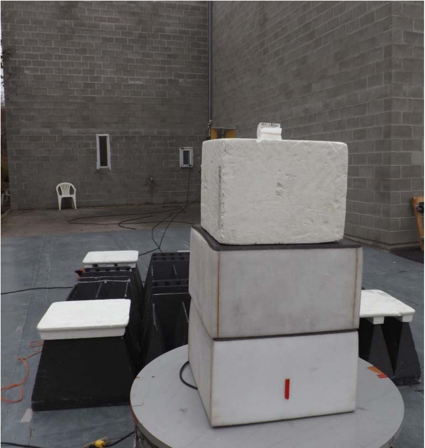
Figure E23.4 – Setup, Radiated Tx Emissions Measurements Above 1000MHz
