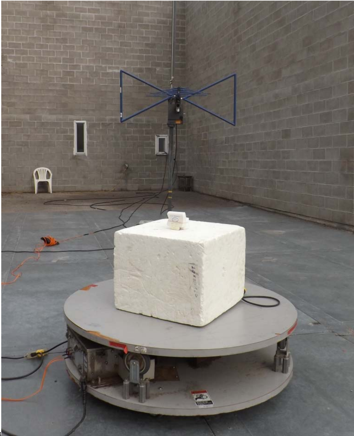
Figure E23.3 – Setup, Radiated Emissions Measurements 30 - 1000MHz
