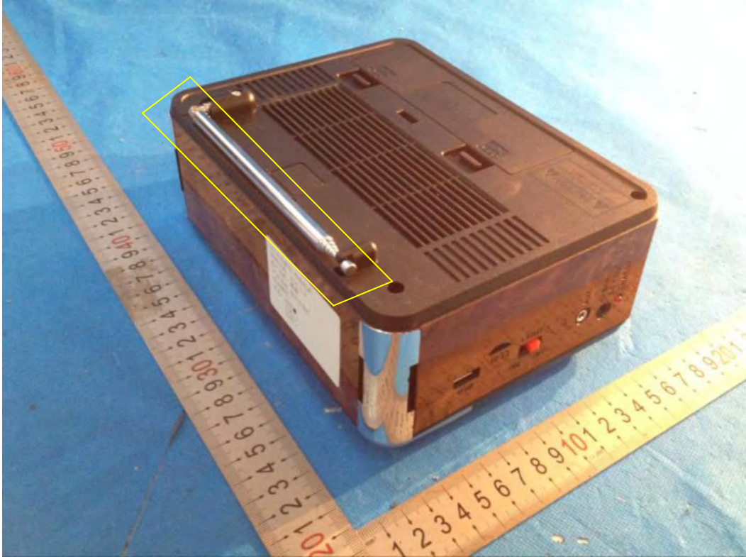
External FM Antenna, length: 60cm
