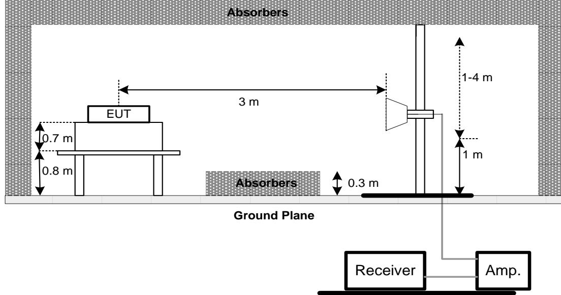
(C) For Radiated Emissions Below 30MHz
