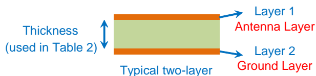
Figure 11. Clarification of PCB Thickness
