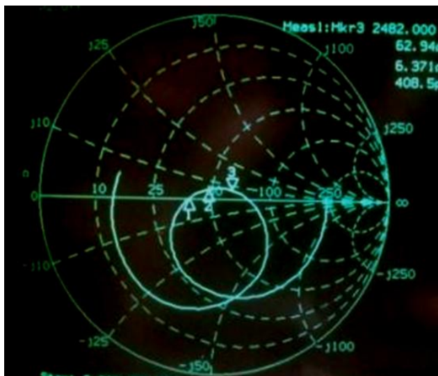
Figure 45. Smith Chart with Real Components
