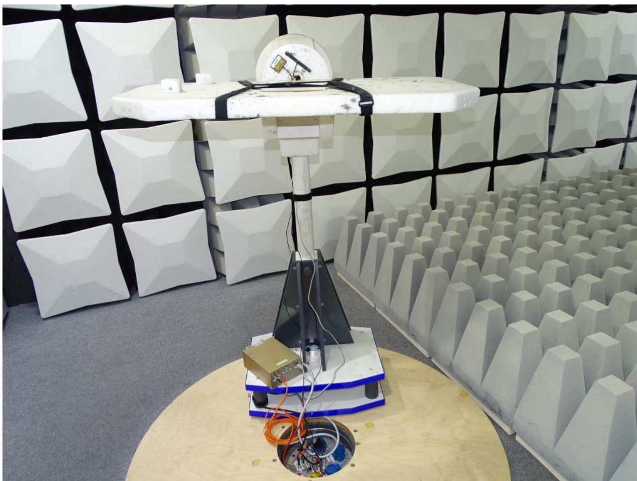
Photo 6: Test setup for radiated measurements above 1 GHz, right side view EUT fixed on EUT-positioning device, fibre optic USB converter near floor
