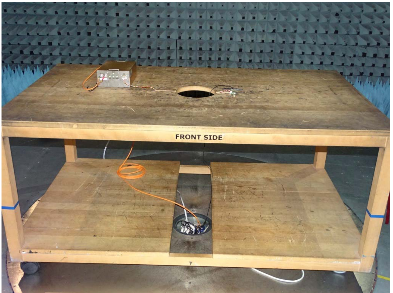
Photo 1: Test setup for radiated measurements below 1 GHz, front side view
