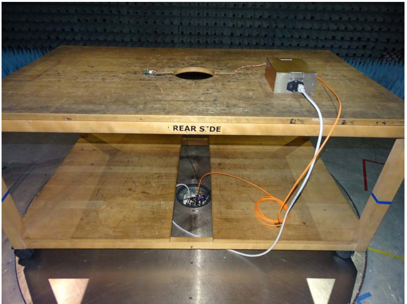
Photo 5: Test setup for radiated measurements below 1 GHz, rear side view
