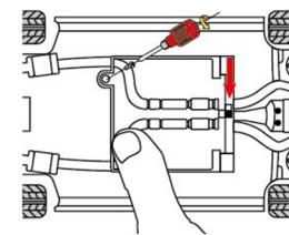
Turn the power switch to the OFF position. Loosen the screw of the battery compartment with a Phillips screwdriver.
