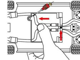
Slide cover up into place. Fasten the screw of the battery compartment. Ensure a tight fit.
