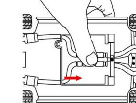
With light pressure on the front end of the battery cover, slide it towards the rear of the vehicle.
