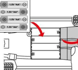
Lift up the battery cover. Replace the batteries following the correct polarities indicated. Close the battery cover.
