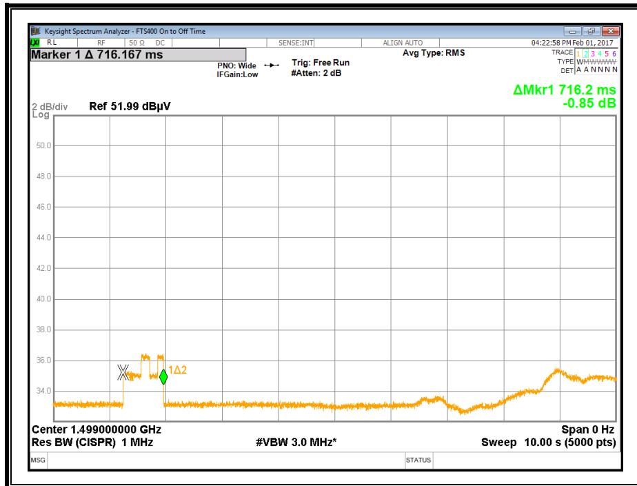
Time denotes total time from button press commanding radar on to button release and radar off. The measured time was 716.2 ms.
