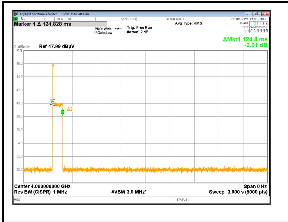
Time denotes total time from button press commanding radar on to button release and radar off. The measured time was 124.8 ms.
