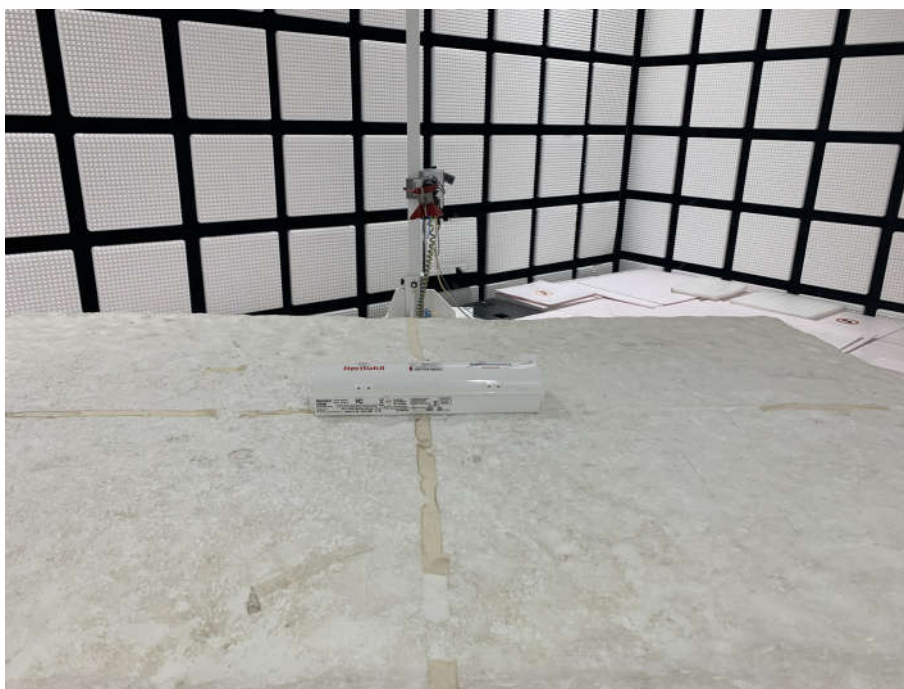
Radiated spurious emission Test Setup-2(Above 1GHz)
