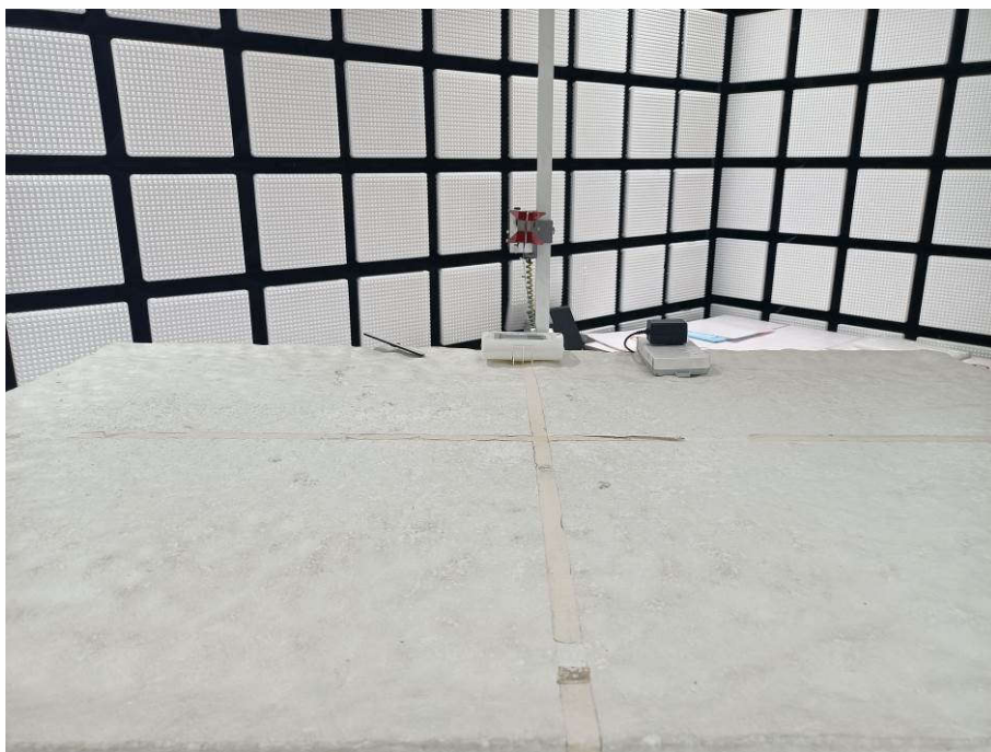
Radiated spurious emission Test Setup-2(Above 1GHz)
