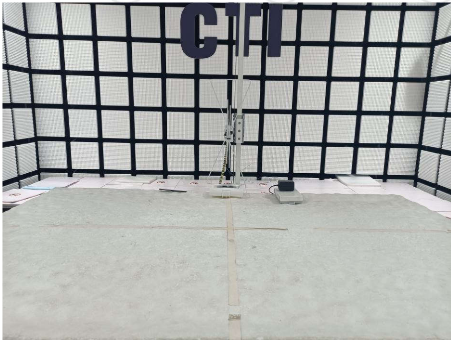
Radiated spurious emission Test Setup-1(Below 1GHz)
