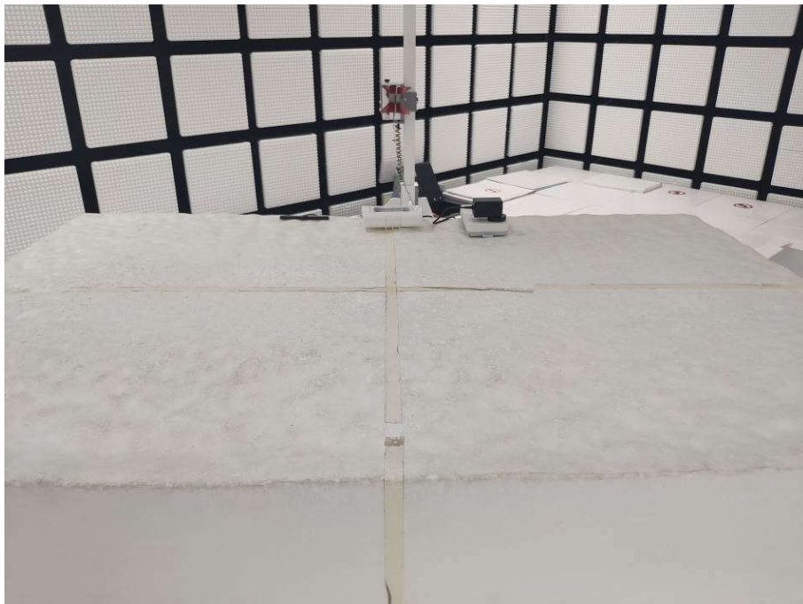
Radiated spurious emission Test Setup-2(Above 1GHz)
