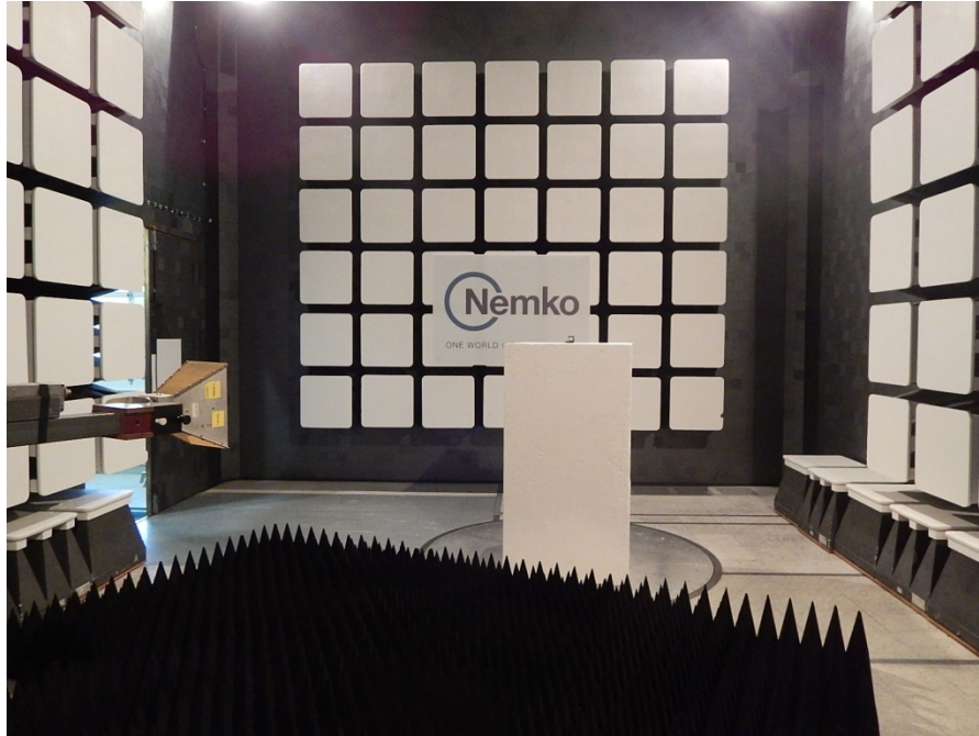
Figure 8.3-24: Radiated spurious (out-of-band) emissions setup photo – above 1 GHz
