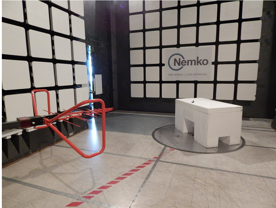
Figure 8.3-22: Radiated spurious (out-of-band) emissions setup photo – 30 to 1000 MHz
