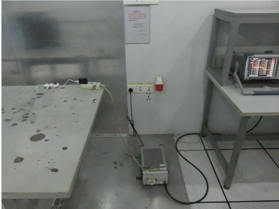
Photo of Conducted Emission Measurement
