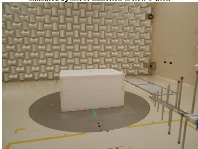
**Radiated Spurious Emission (Above 1 GHz) / Band Edge Measurement**
