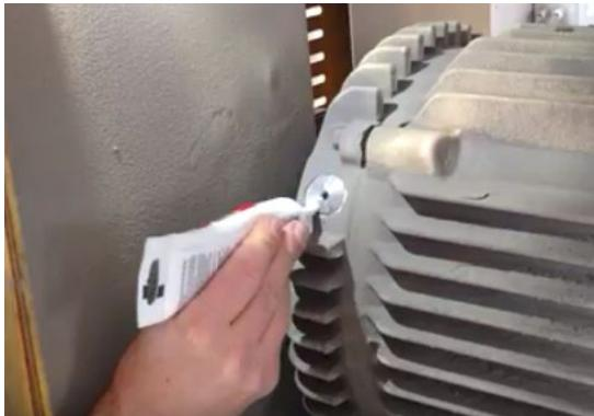
7. Hand-tighten the sensor to machine (do not use tools).
