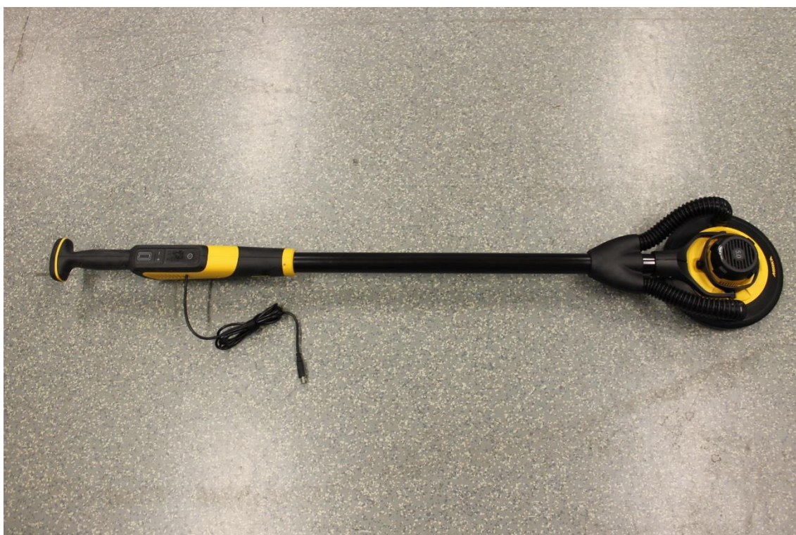
Photograph 2. The EUT 2 sample with test setup cable for radiated emission tests.
