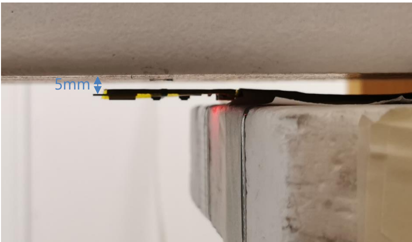
Figure 12 Back Test Position, RF Energy Coupling Enhancement, 5mm separation distance
