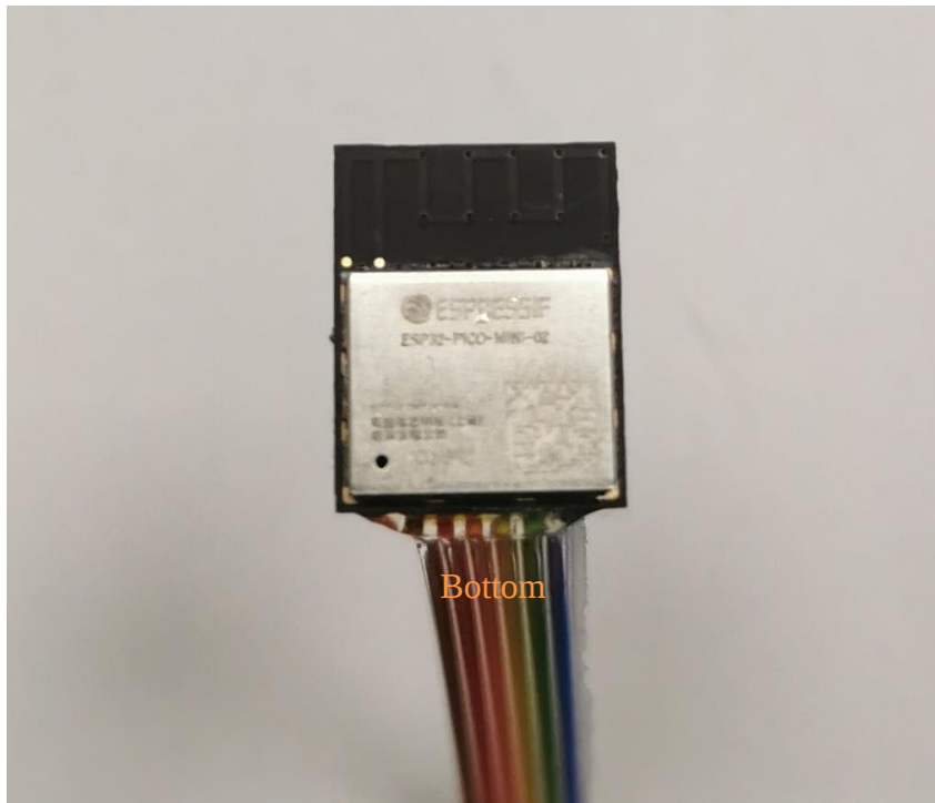
Figure 4 ESP32-PICO-MINI-02 Module attached with wires
