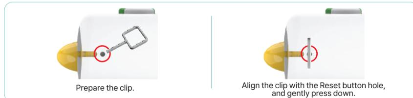
① Using the pointed end of a clip, gently press the Reset button located inside the small hole. (The clip is not included in this package.)
