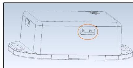
Next, gently double tap the device until a blue light appears, then double tap again. The blue light will begin flashing, indicating the device is in "access point mode" and is ready to pair with your mobile phone using the Trakkit App. The user should notice a solid blue light and flashing yellow light to indicate the device is in "access point mode". Use the mobile app to finalize the activation of your device.
