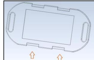
Once open, carefully insert AAA batteries one at a time, paying close attention to the positive and negative contact ends. Replace bottom cover in a way such that the grooves cover the batteries.
