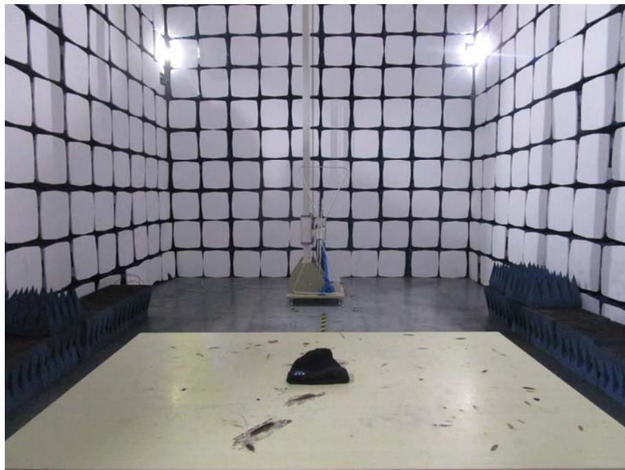
**Radiation Emission Test Setup (Above 1GHz)**
