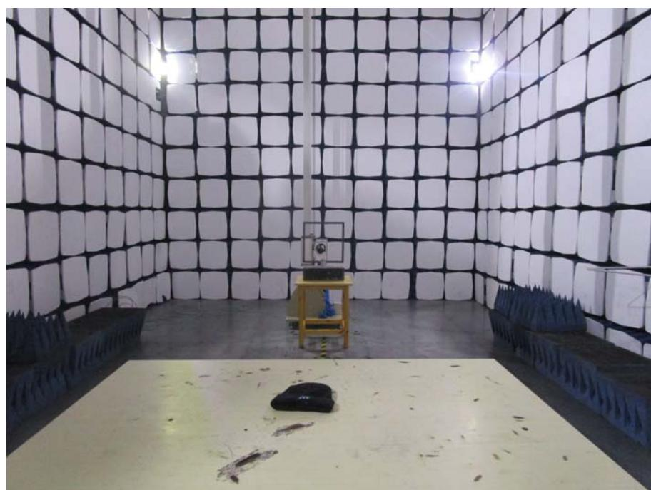
**Radiation Emission Test Setup (30MHz to 1GHz)**
