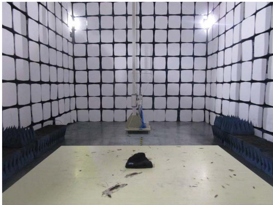
**Radiation Emission Test Setup (Above 1GHz)**
