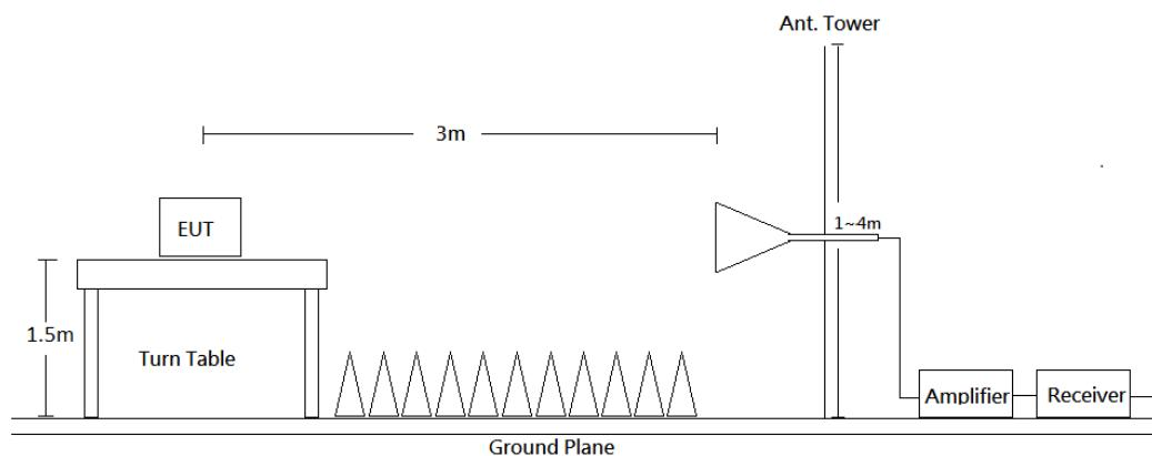
Radiated emission tests were performed in the 3 meters chamber test site, using the setup accordance with the ANSI C63.10-2013. The specification used was the FCC 15.205, FCC 15.209, FCC 15.249 and RSS-GEN, RSS-210 limits.
