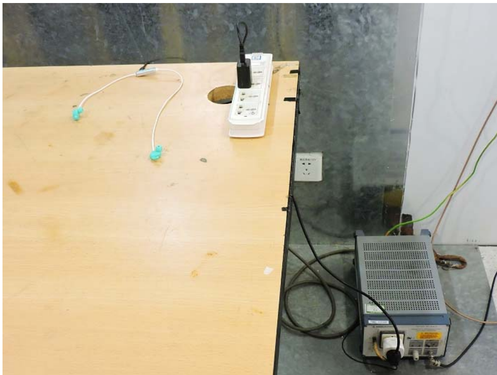
Conducted Emission Test Setup:
