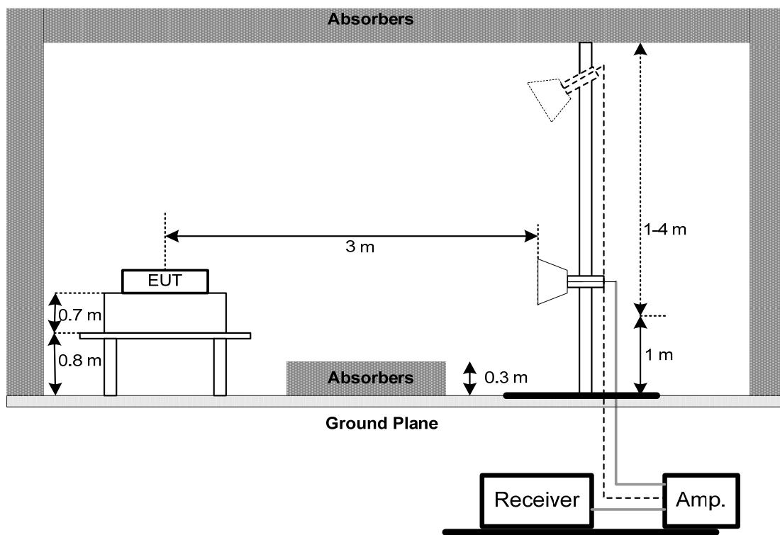
(C) For radiated emissions below 30MHz
