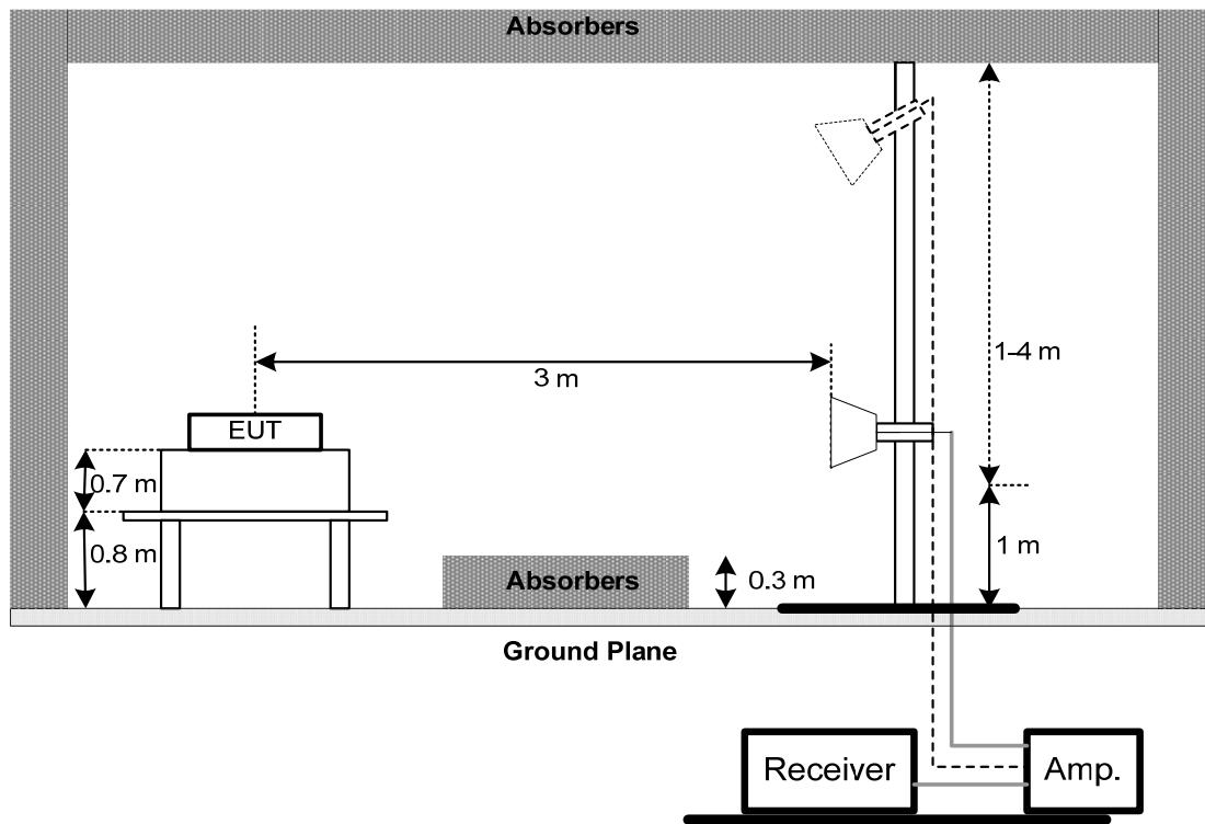
(C) For radiated emissions below 30MHz
