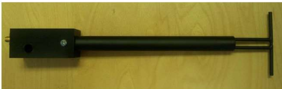
Figure 1 – MVG COMOSAR Validation Dipole
