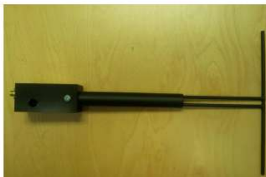
Figure 1 – MVG COMOSAR Validation Dipole
