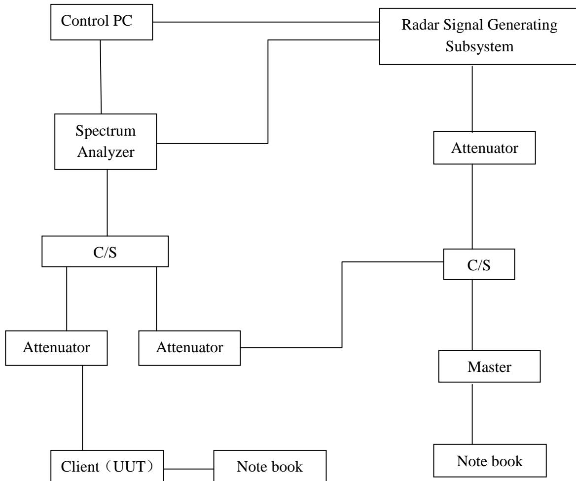
The UUT is a UNII device operating in client mode without radar detection. The radar test signals are injected into the master device.
