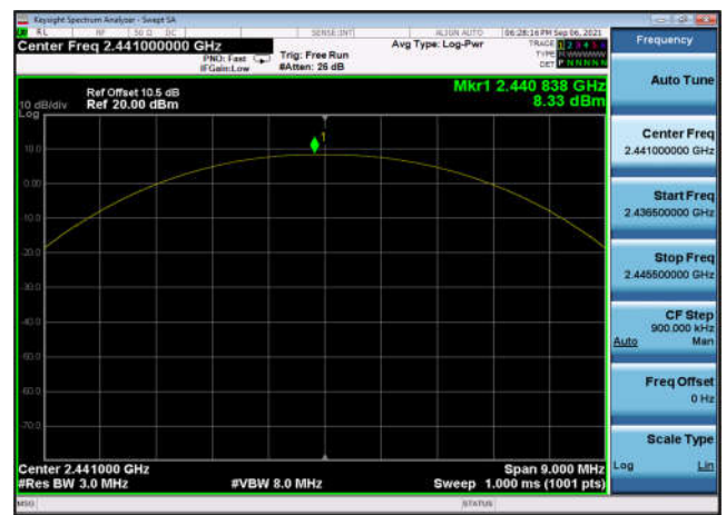
Output Power: DQPSK,2402MHz,2DH5
