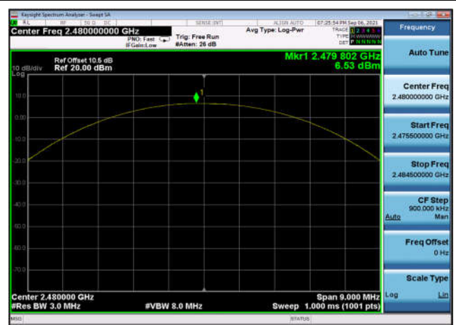
Output Power: DQPSK,2480MHz,2DH5
