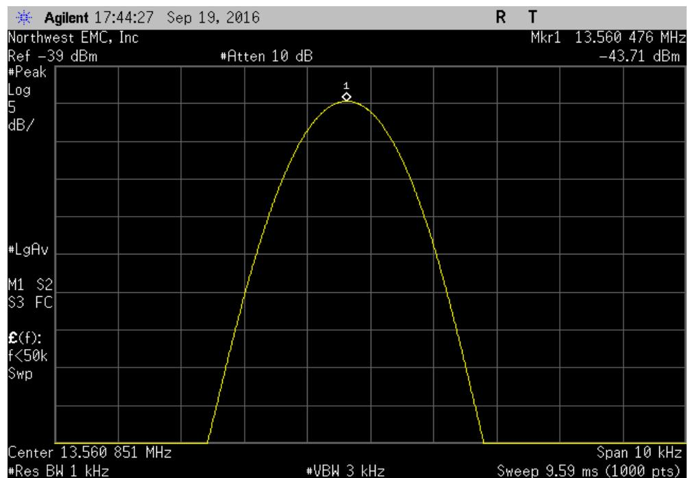
RFID, 13.56 MHz, Temperature: +20°, Startup
