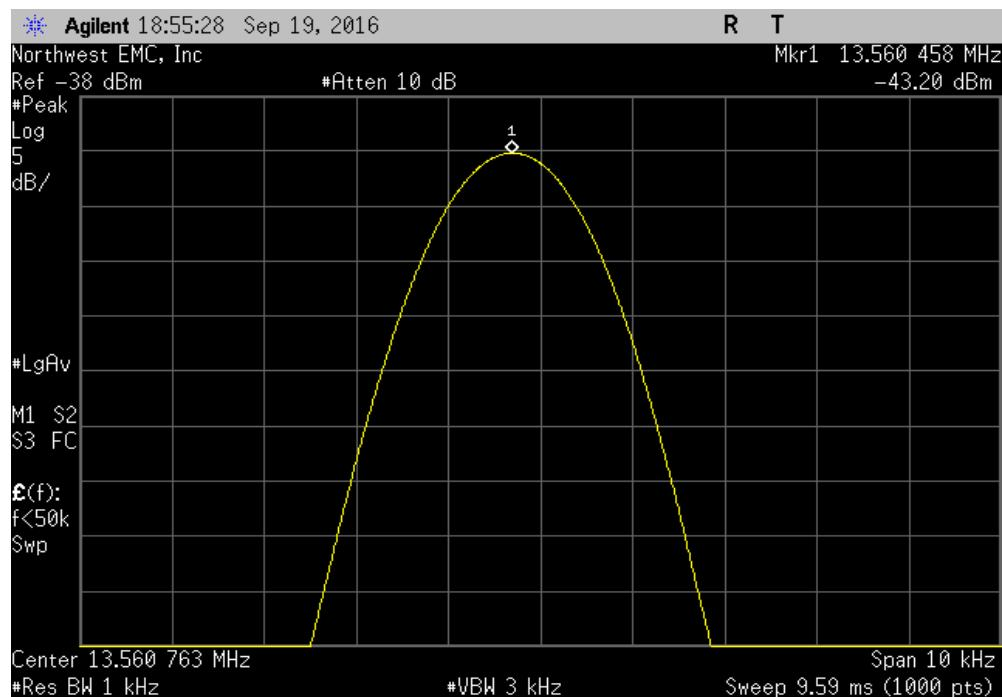
RFID, 13.56 MHz, Temperature: +40°, Startup
