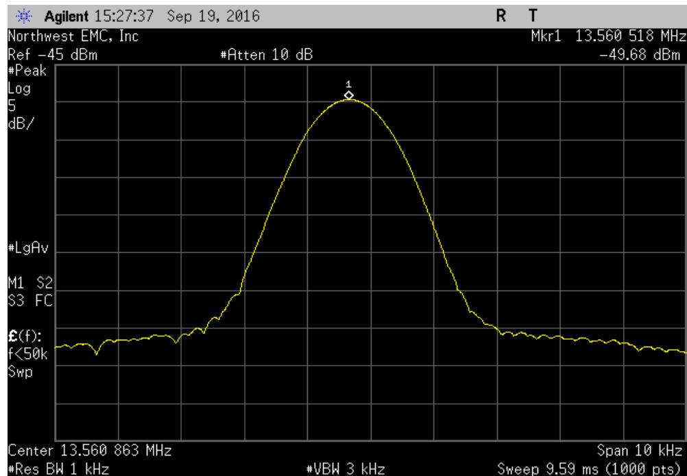
RFID, 13.56 MHz, Temperature: -10°, Startup
