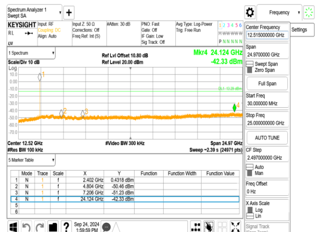
Spurious Emission_BLE 2M_LowCH00-2402MHz
