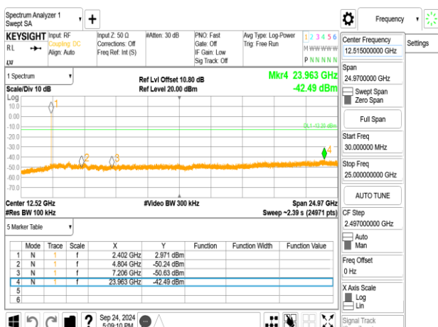
Spurious Emission_BLE 125k_LowCH00-2402MHz
