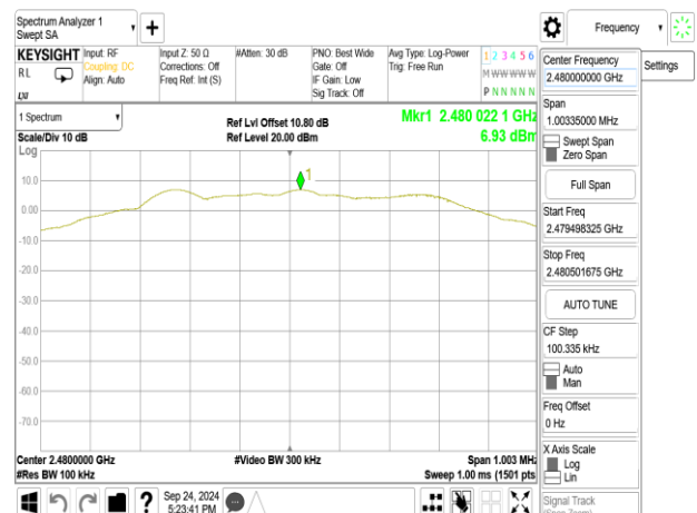
Reference Level_BLE 500k_HighCH39-2480MHz
