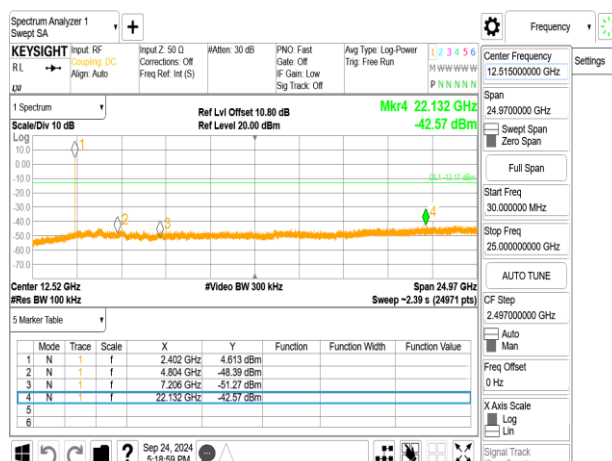
Spurious Emission_BLE 500k_LowCH00-2402MHz
