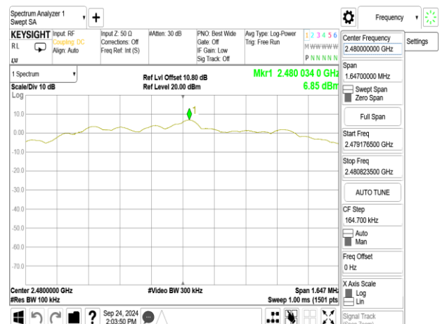
Reference Level_BLE 2M_HighCH39-2480MHz
