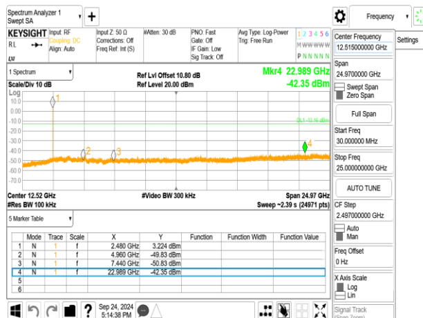
Spurious Emission_BLE 500k_LowCH00-2402MHz
