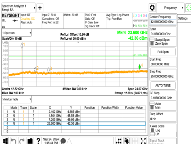
Spurious Emission_BLE 1M_LowCH00-2402MHz
