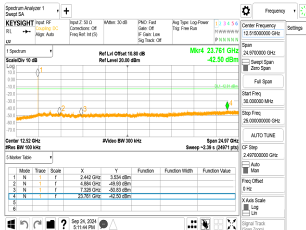
Spurious Emission_BLE 125k_HighCH39-2480MHz
