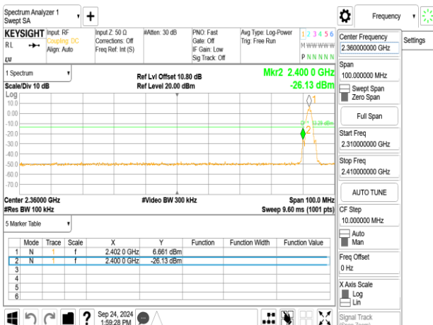
Band Edge_BLE 2M_LowCH00-2402MHz
