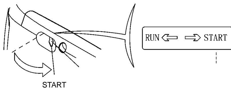
**3. Pull the starter grip until resistance is felt then pull the starter grip briskly toward the arrow as shown below.**
