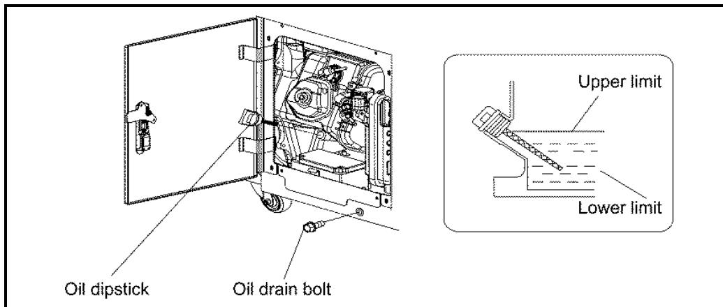
Figure 8 Oil level schematic diagram
