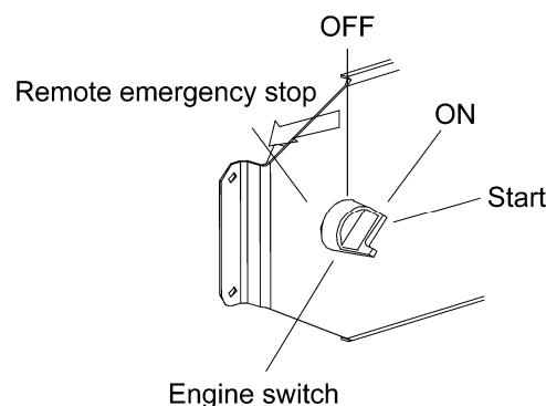
Figure 26 Remote stop in remote start status
