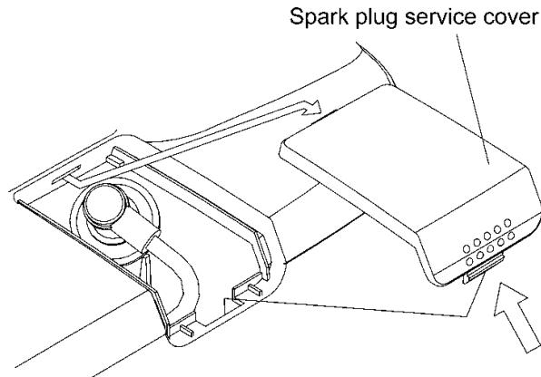
2. Remove the spark plug cap.
