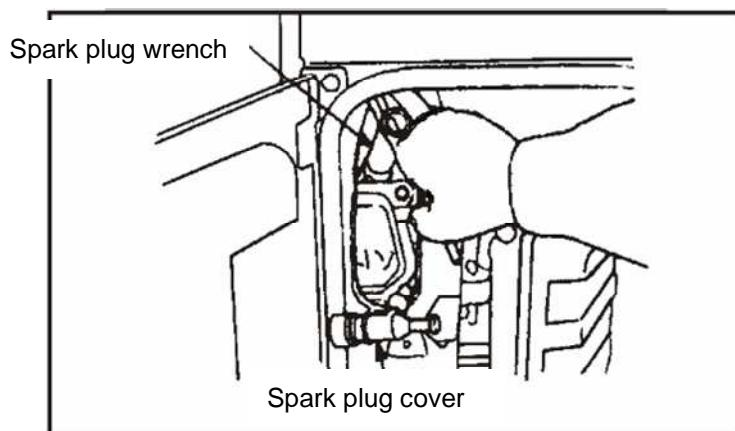
Figure 28 Dismantle the spark plug
