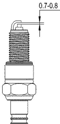
Figure 29 Measure the clearance of spark plug
