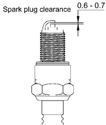
7. Install the spark plug carefully, by hand, to avoid cross-threading.
