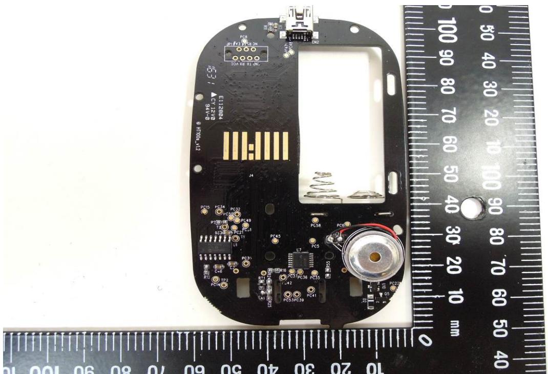
**Internal View of EUT – 1 (Model: HT100-B)**
