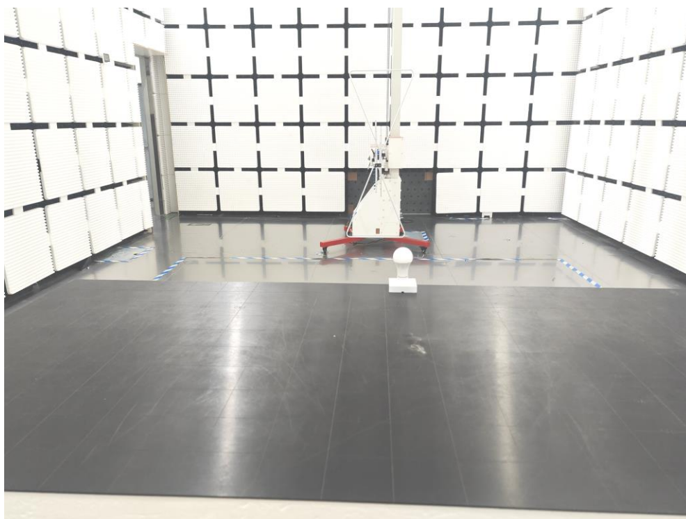
Photo of Radiated Emission test
