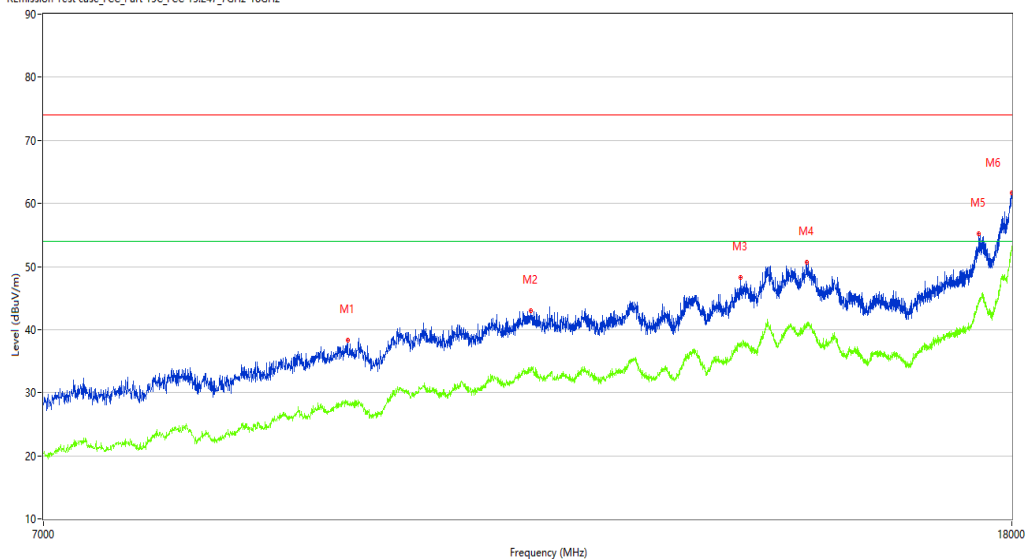
REmission Test case_FCC_Part 15C_FCC 15.247_7GHz-18GHz
