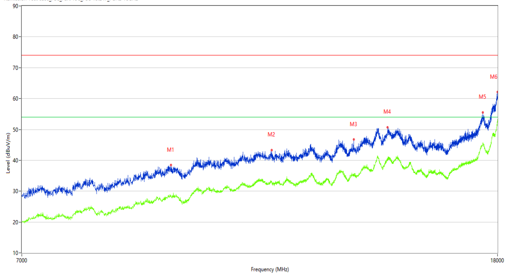
REmission Test case_FCC_Part 15C_FCC 15.247_7GHz-18GHz
