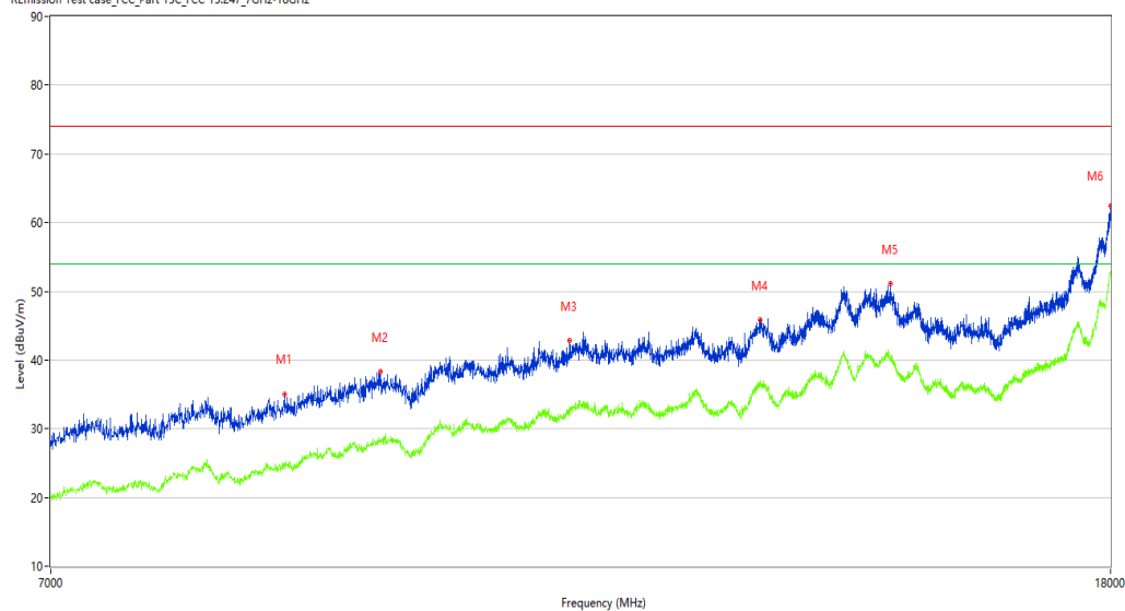
REmission Test case_FCC_Part 15C_FCC 15.247_7GHz-18GHz
