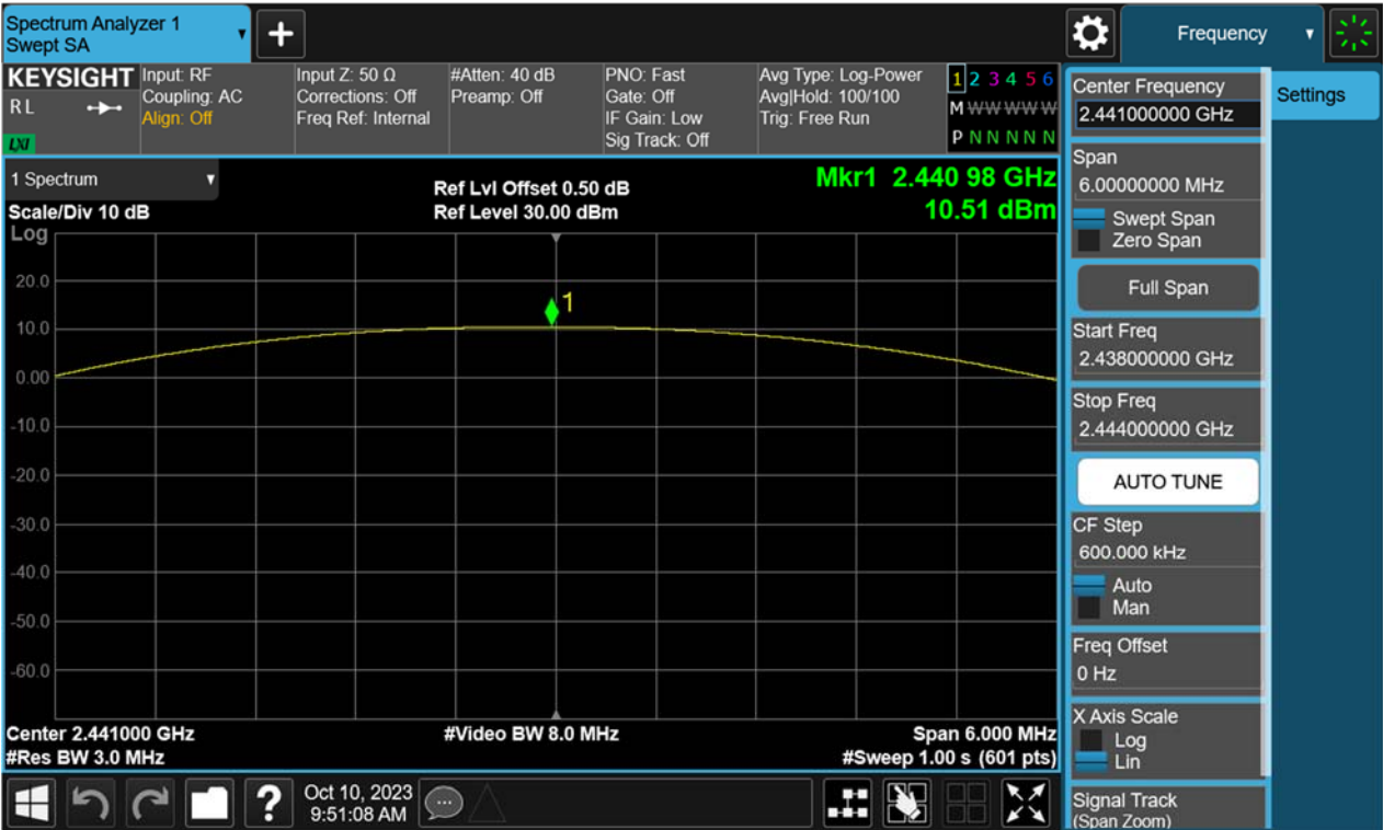
Figure 2: Maximum Peak Output Power, 2441MHz, GFSK
