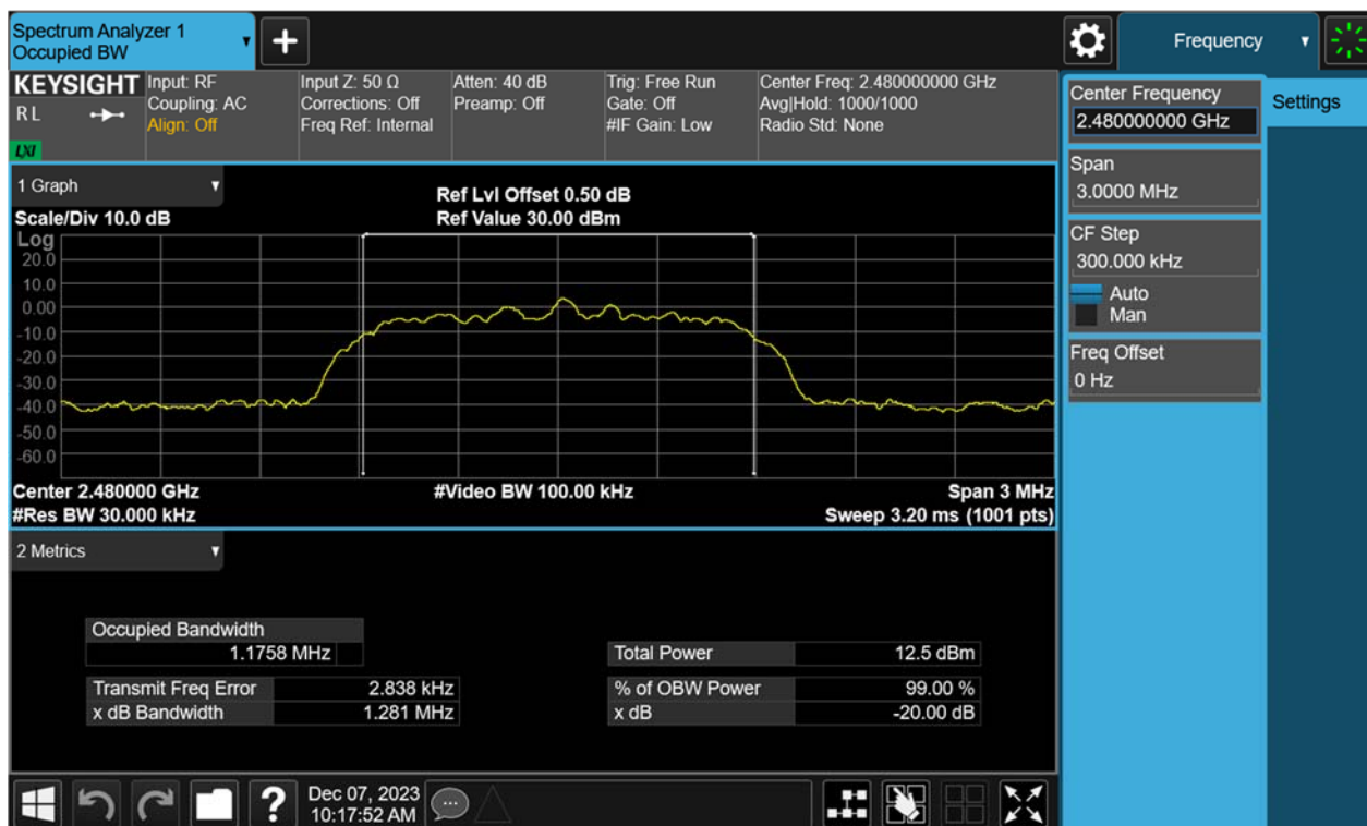
Figure 15: 20dB Bandwidth and 99% Bandwidth, 2480MHz, \pi/4 -DQPSK
