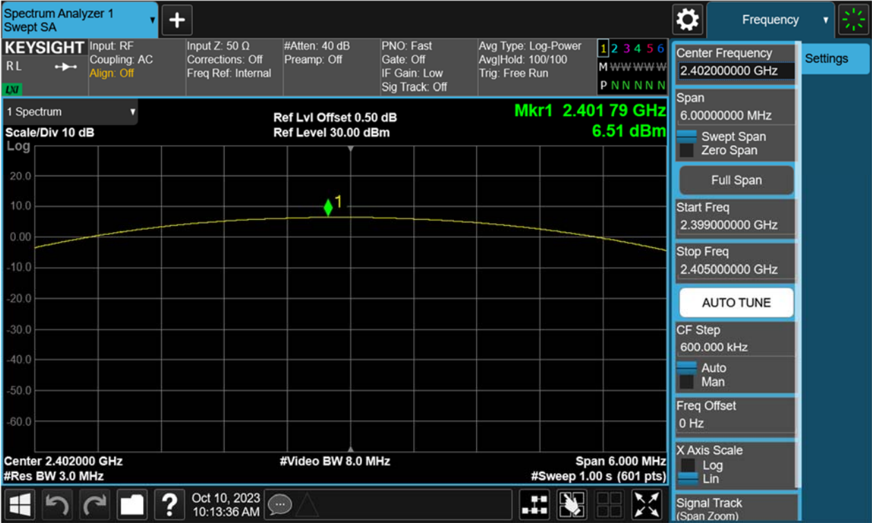
Figure 8: Maximum Peak Output Power, 2441MHz, 8-DPSK
