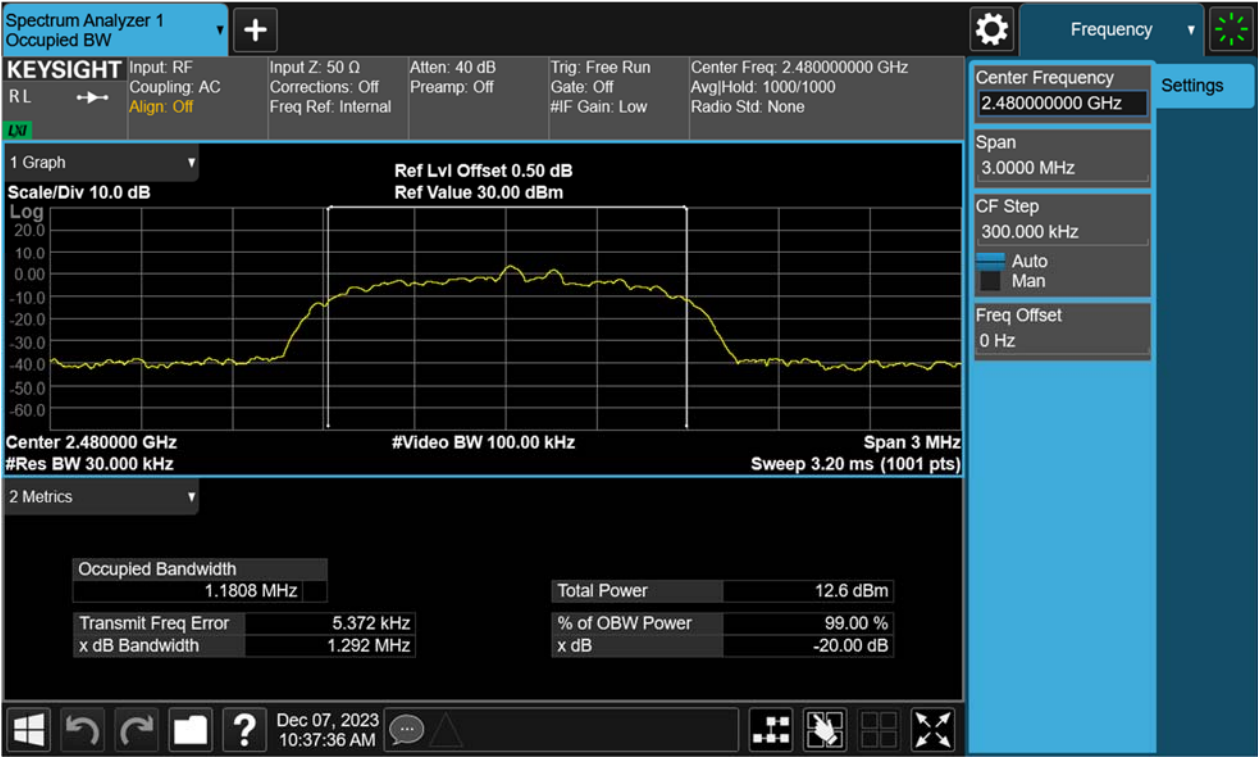
Figure 18: 20dB Bandwidth and 99% Bandwidth, 2480MHz, 8-DPSK
