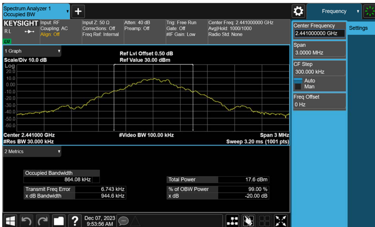
Figure 11: 20dB Bandwidth and 99% Bandwidth, 2441MHz, GFSK
