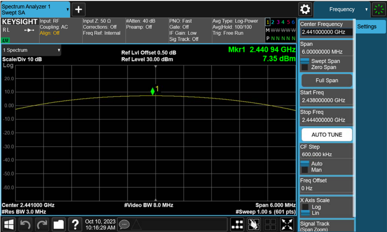
Figure 8: Maximum Peak Output Power, 2441MHz, 8-DPSK
