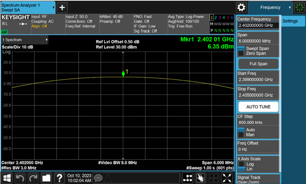
Figure 4: Maximum Peak Output Power, 2402MHz, \pi/4 -DQPSK
