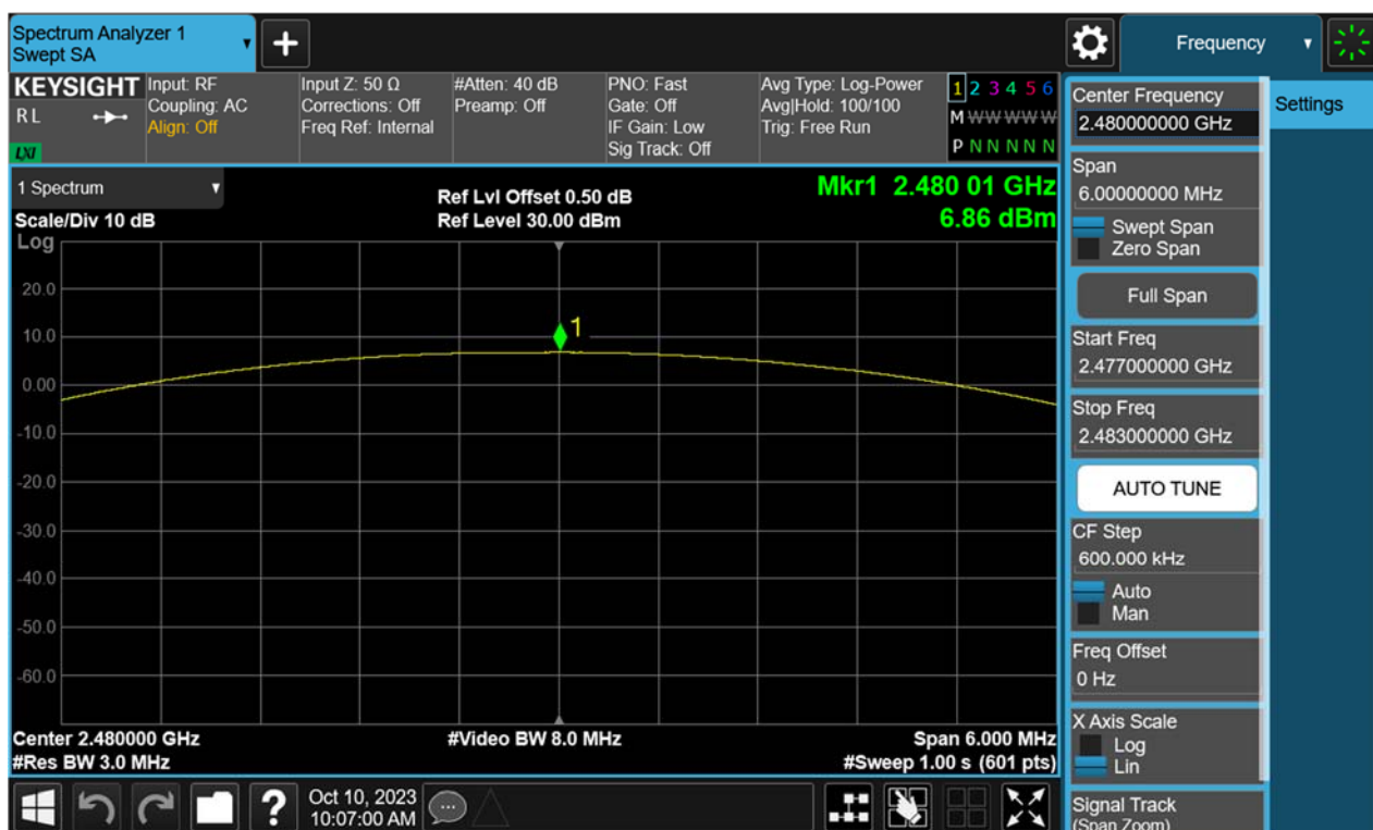
Figure 6: Maximum Peak Output Power, 2480MHz, \pi/4 -DQPSK
