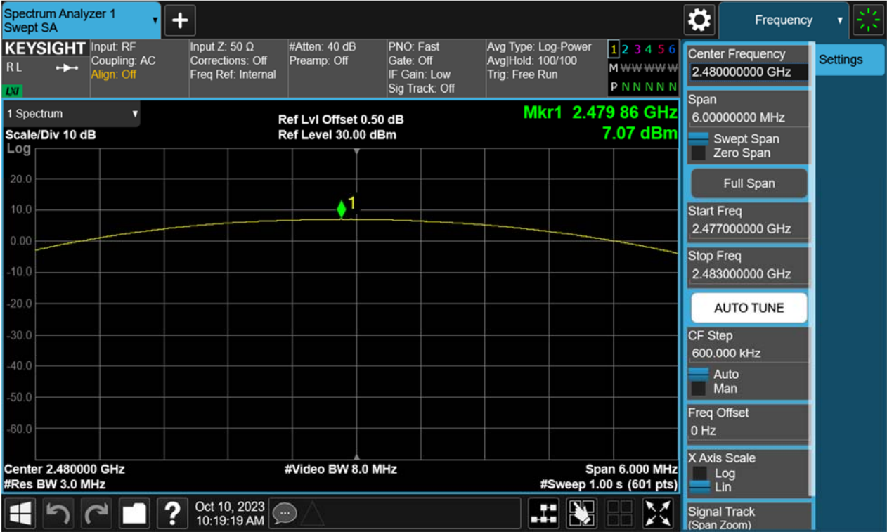
Figure 9: Maximum Peak Output Power, 2480MHz, 8-DPSK
