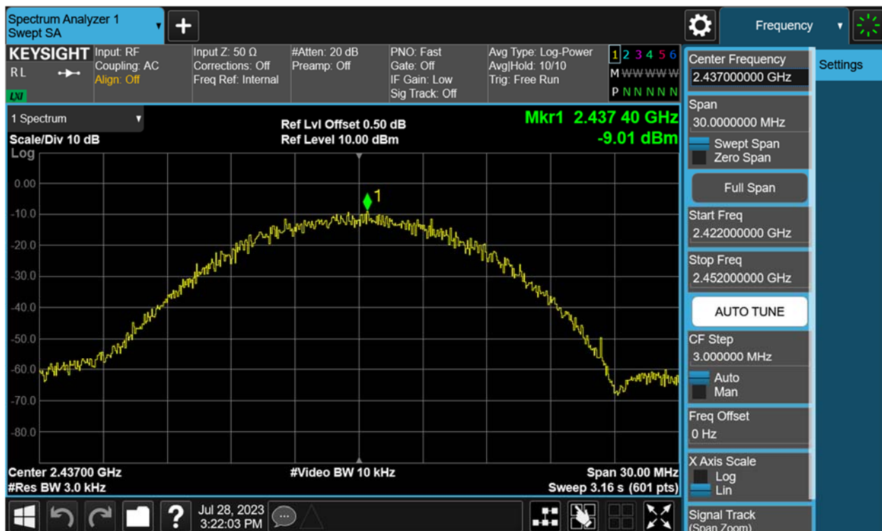
Figure 14: Power Spectral Density, 802.11b, 2437MHz
