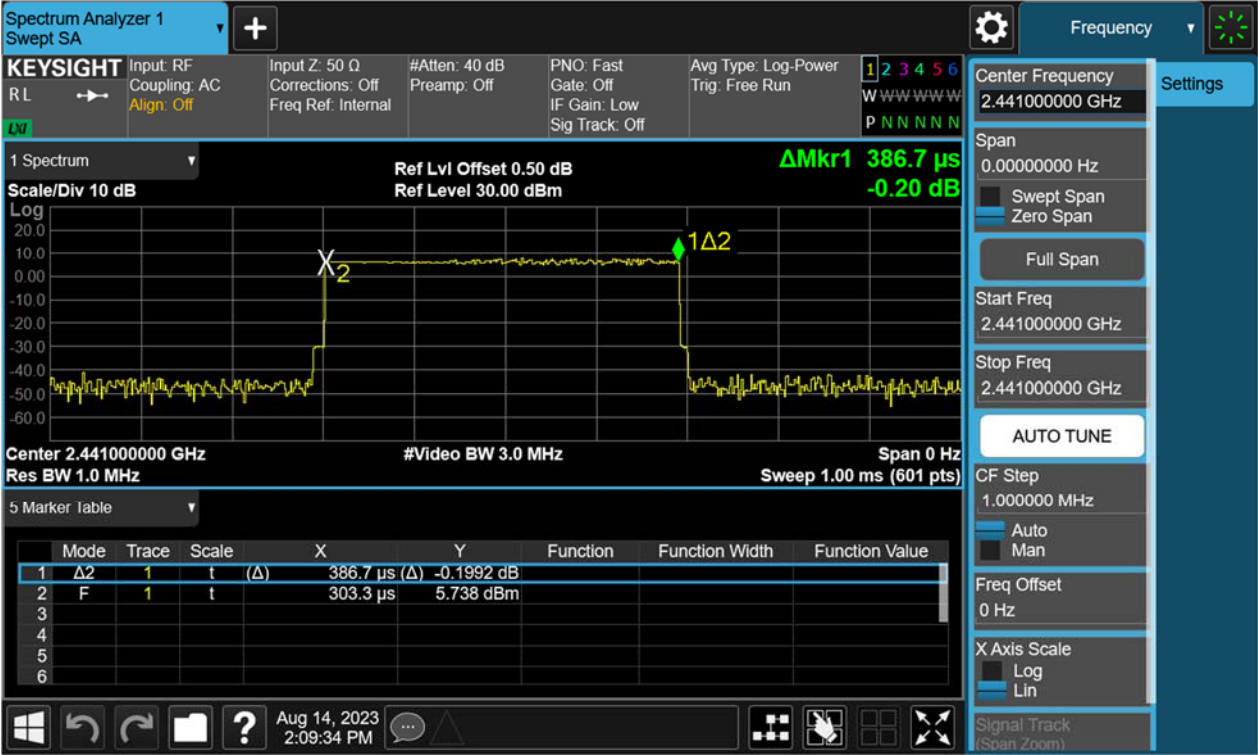
Figure 44: Time of Occupancy, 2441MHz, 8-DPSK DH3
