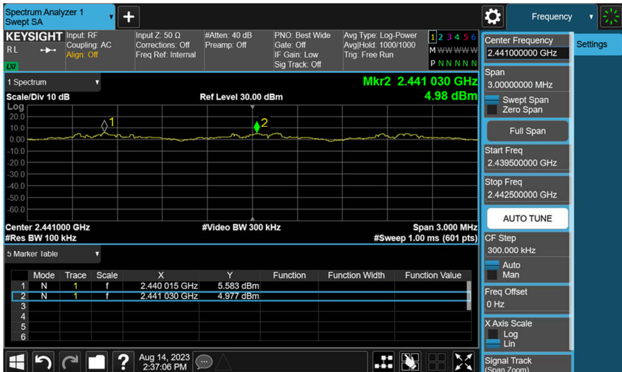
Figure 32: Hopping Frequency Separation, Hopping Mode, \pi/4 -DQPSK
