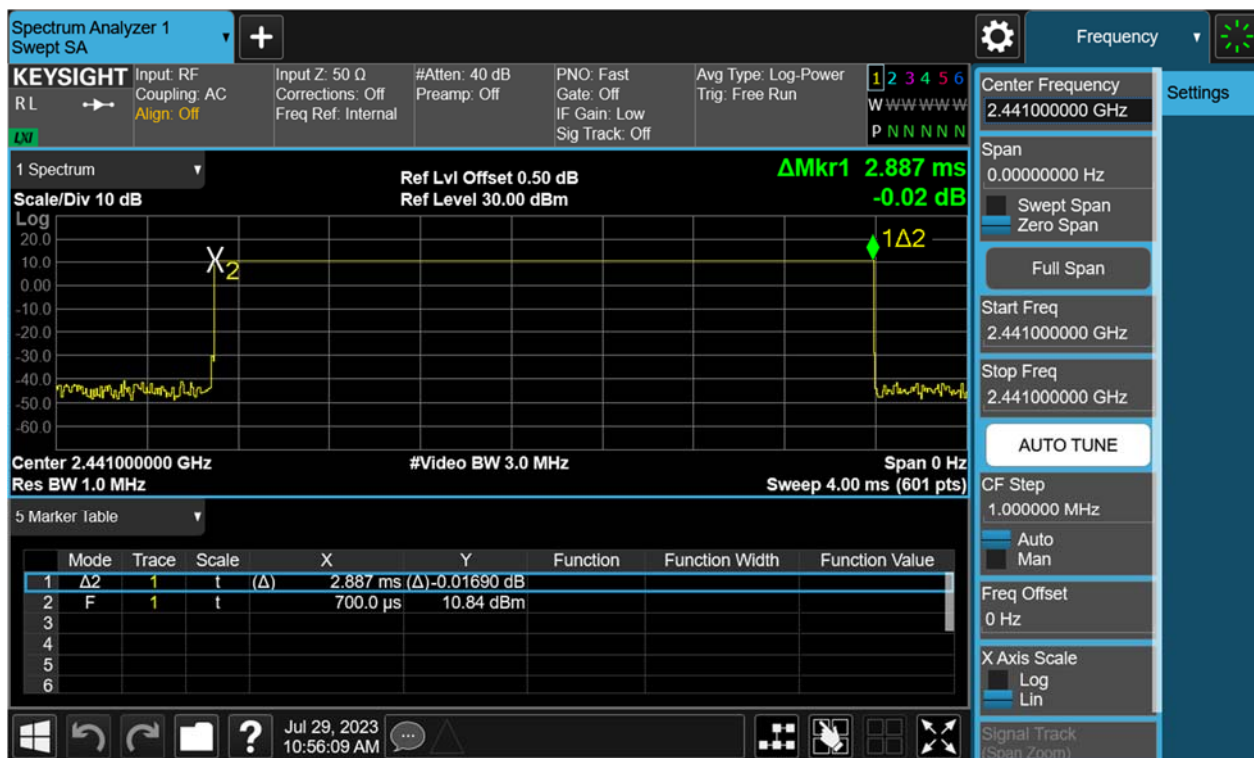
Figure 40: Time of Occupancy, 2441MHz, \pi/4 -DQPSK DH1
