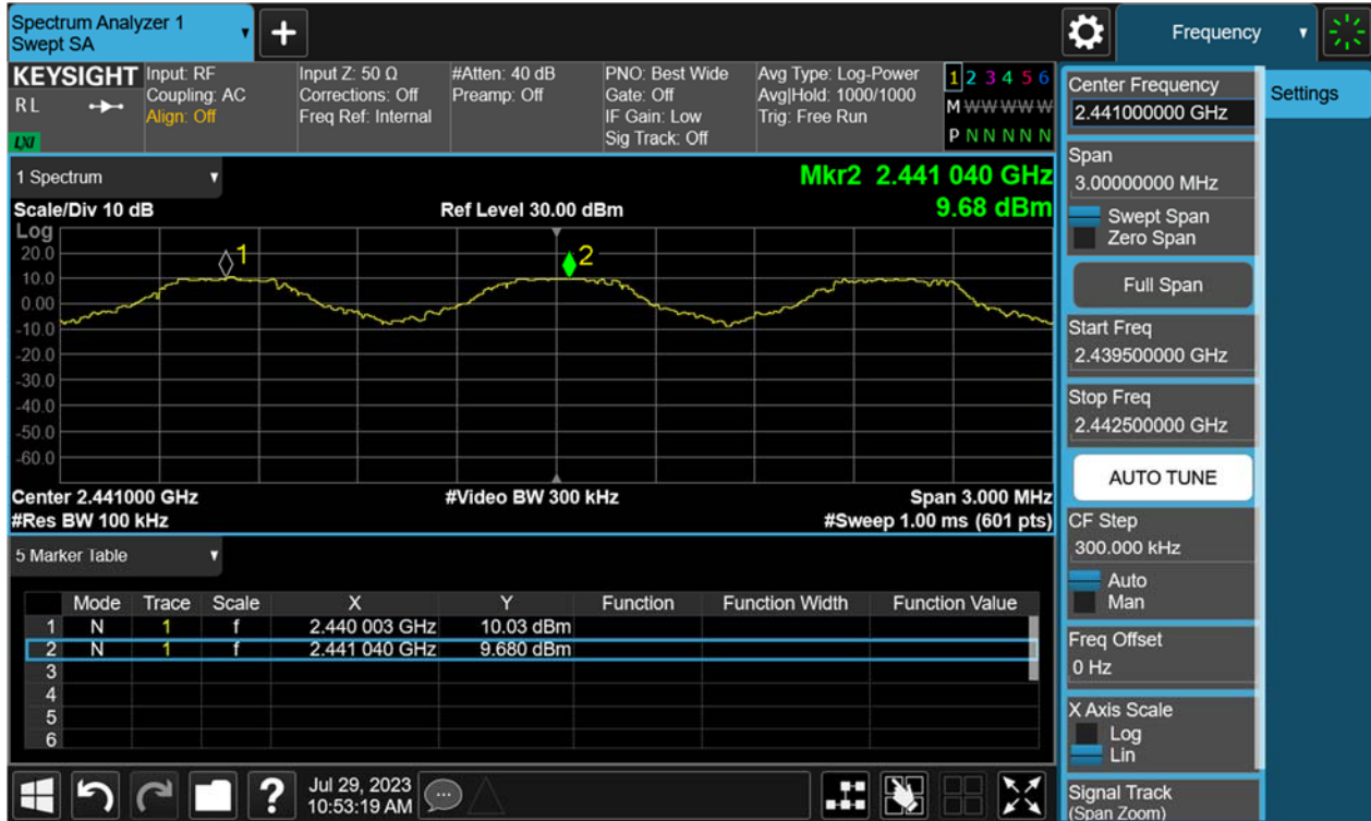
Figure 32: Hopping Frequency Separation, Hopping Mode, \pi/4 -DQPSK
