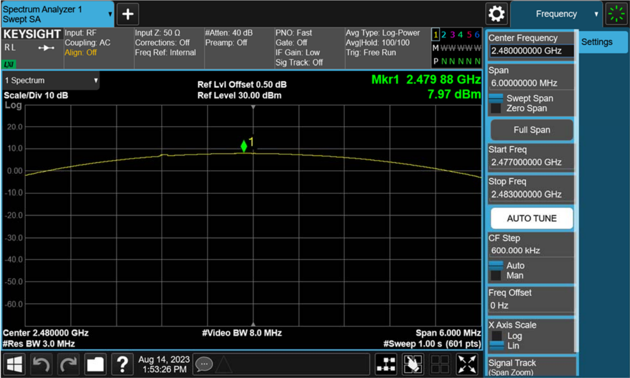
Figure 9: Maximum Peak Output Power, 2480MHz, 8-DPSK
