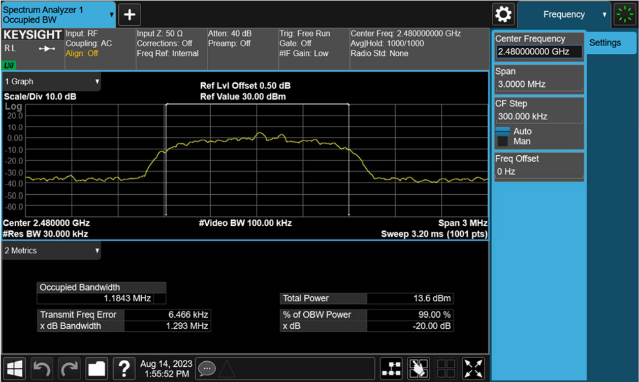
Figure 18: 20dB Bandwidth, 2480MHz, 8-DPSK
