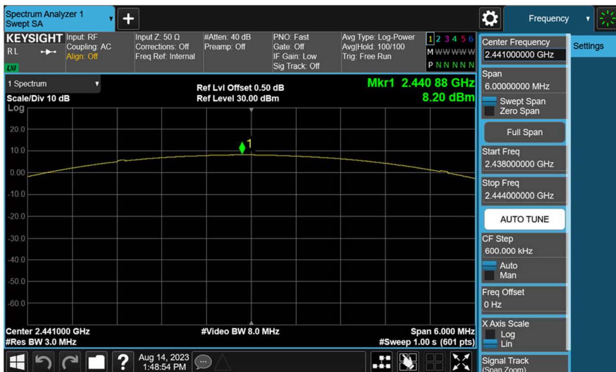
Figure 8: Maximum Peak Output Power, 2441MHz, 8-DPSK
