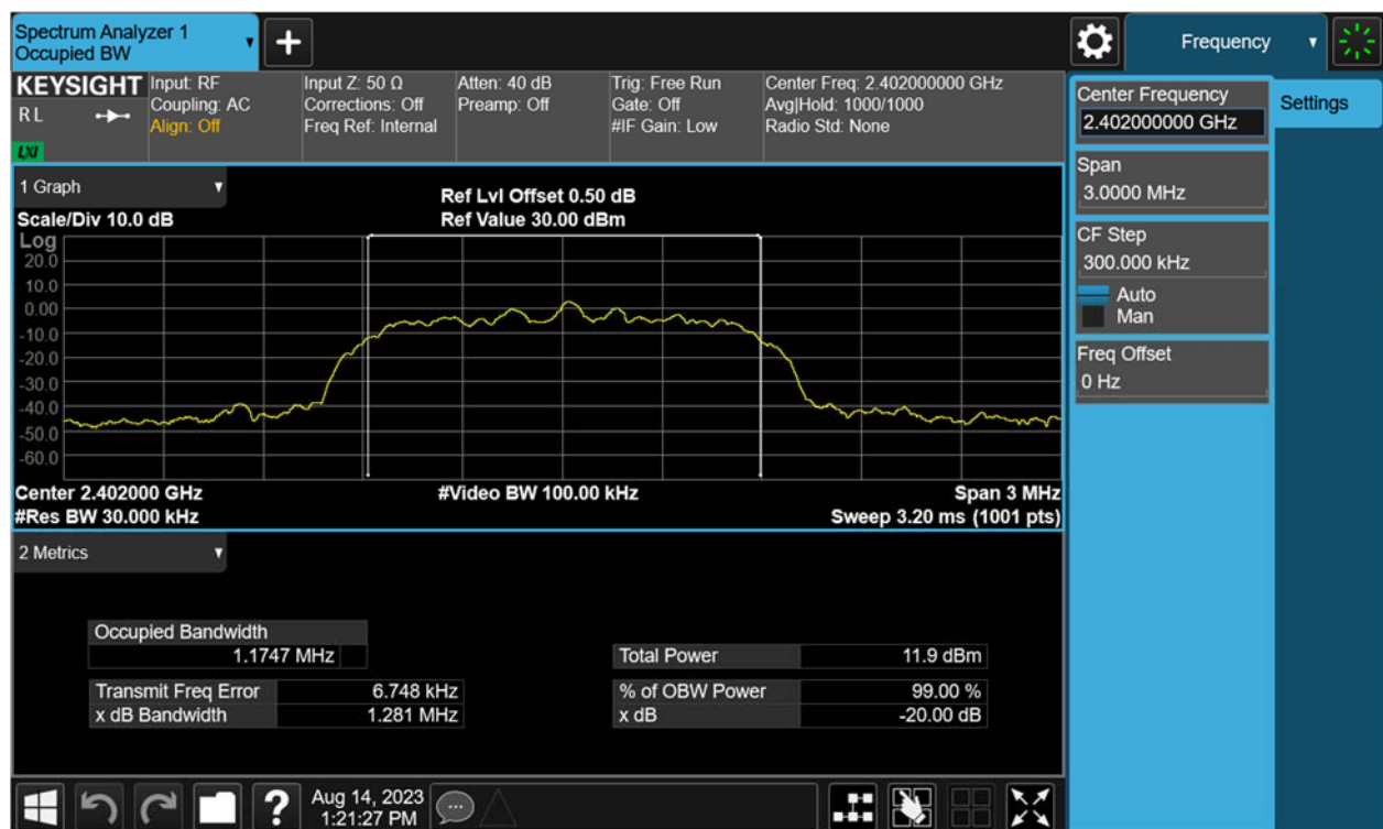
Figure 13: 20dB Bandwidth, 2402MHz, \pi/4 -DQPSK
