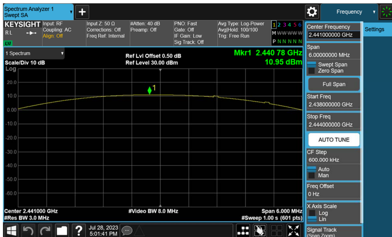
Figure 2: Maximum Peak Output Power, 2441MHz, GFSK
