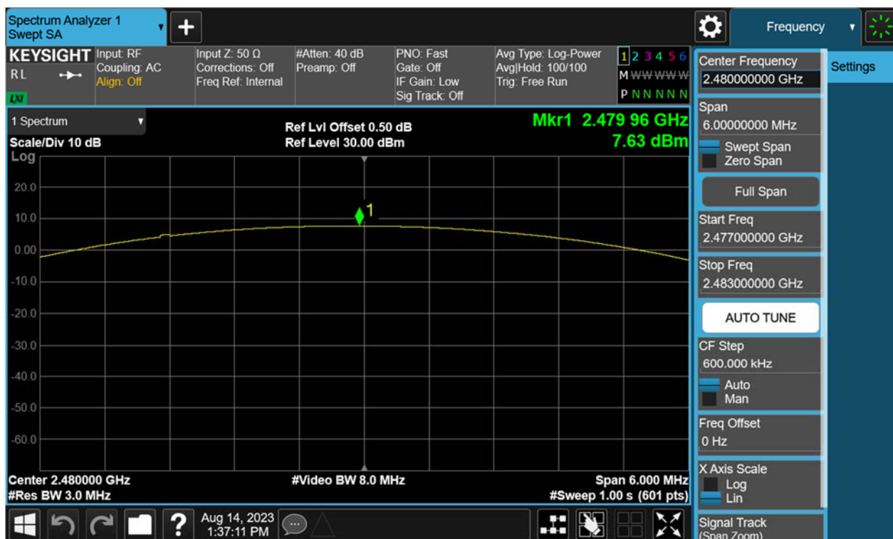
Figure 6: Maximum Peak Output Power, 2480MHz, \pi/4 -DQPSK
