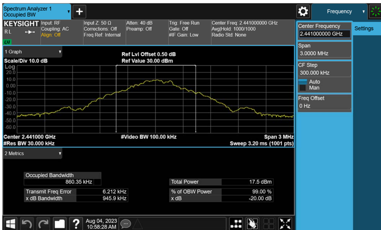
Figure 11: 20dB Bandwidth, 2441MHz, GFSK
