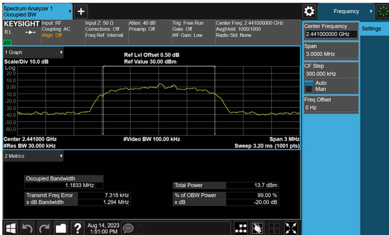
Figure 17: 20dB Bandwidth, 2441MHz, 8-DPSK
