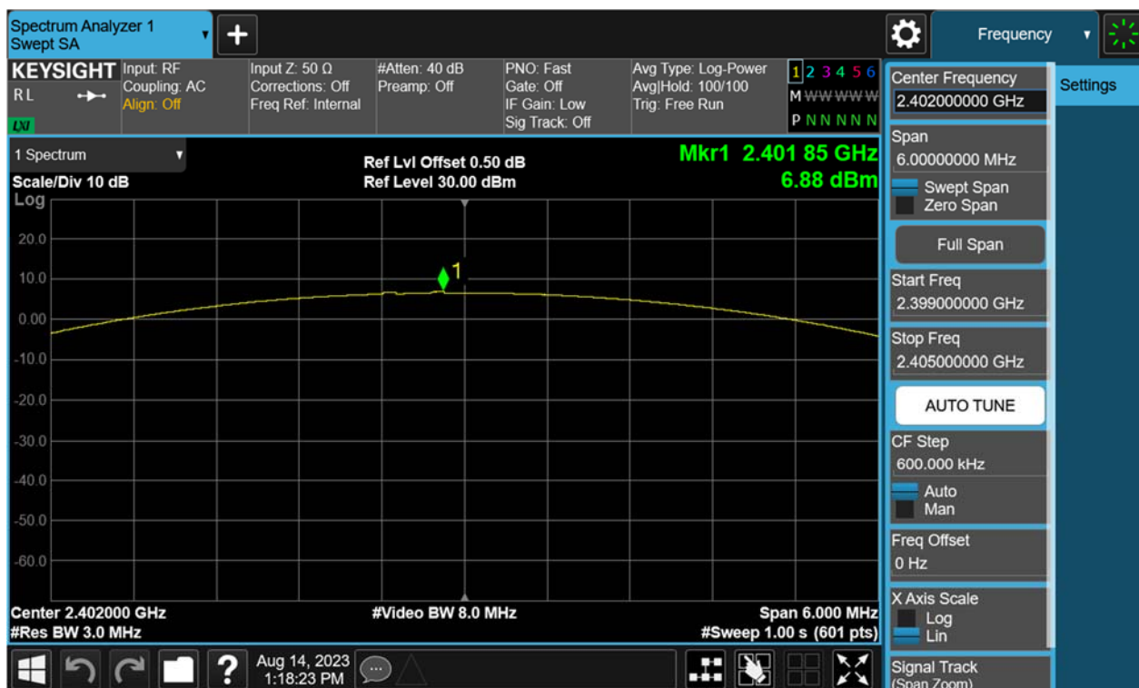
Figure 4: Maximum Peak Output Power, 2402MHz, \pi/4 -DQPSK
