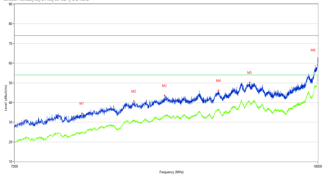
REmission Test case_FCC_Part 15C_FCC 15.247_7GHz-18GHz
