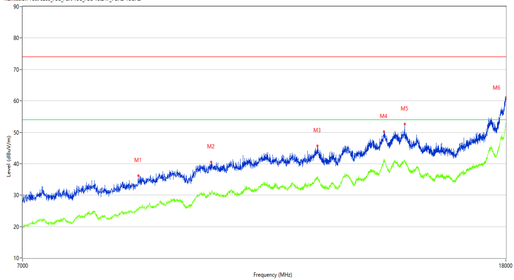
R/Emission Test case_FCC_Part 15C_FCC 15.247_7GHz-18GHz
