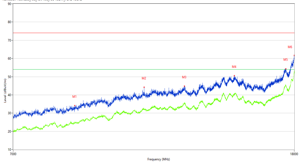
REmission Test case_FCC_Part 15C_FCC 15.247_7GHz-18GHz
