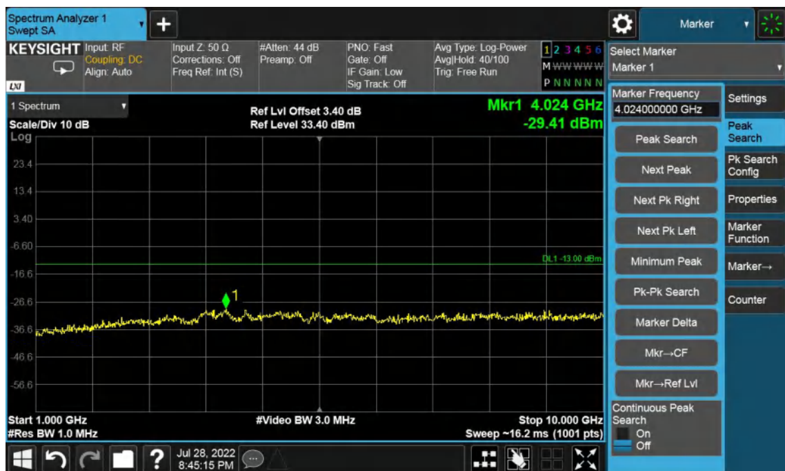
High Channel-5MHz Bandwidth-1GHz to 10GHz
