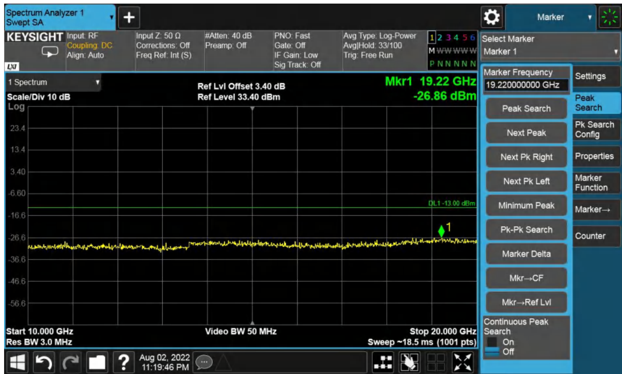
Low Channel-1.4MHz Bandwidth-10GHz to 20GHz
