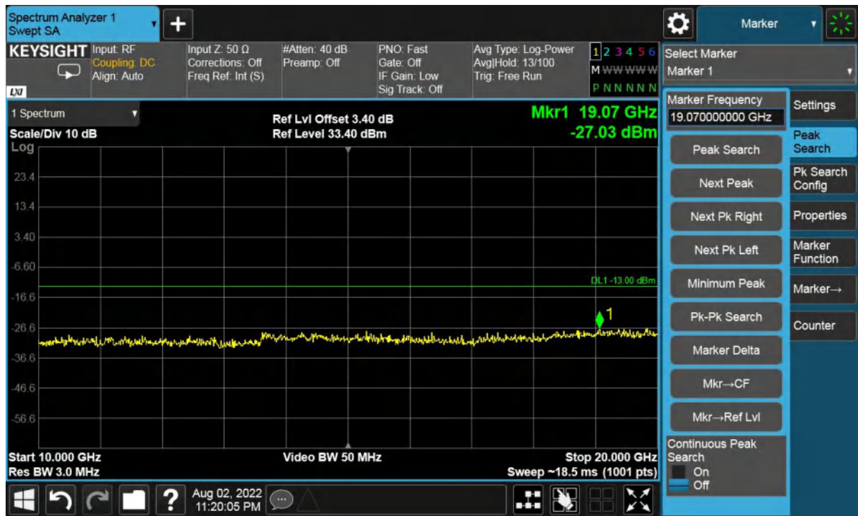
High Channel-5MHz Bandwidth-10GHz to 20GHz
