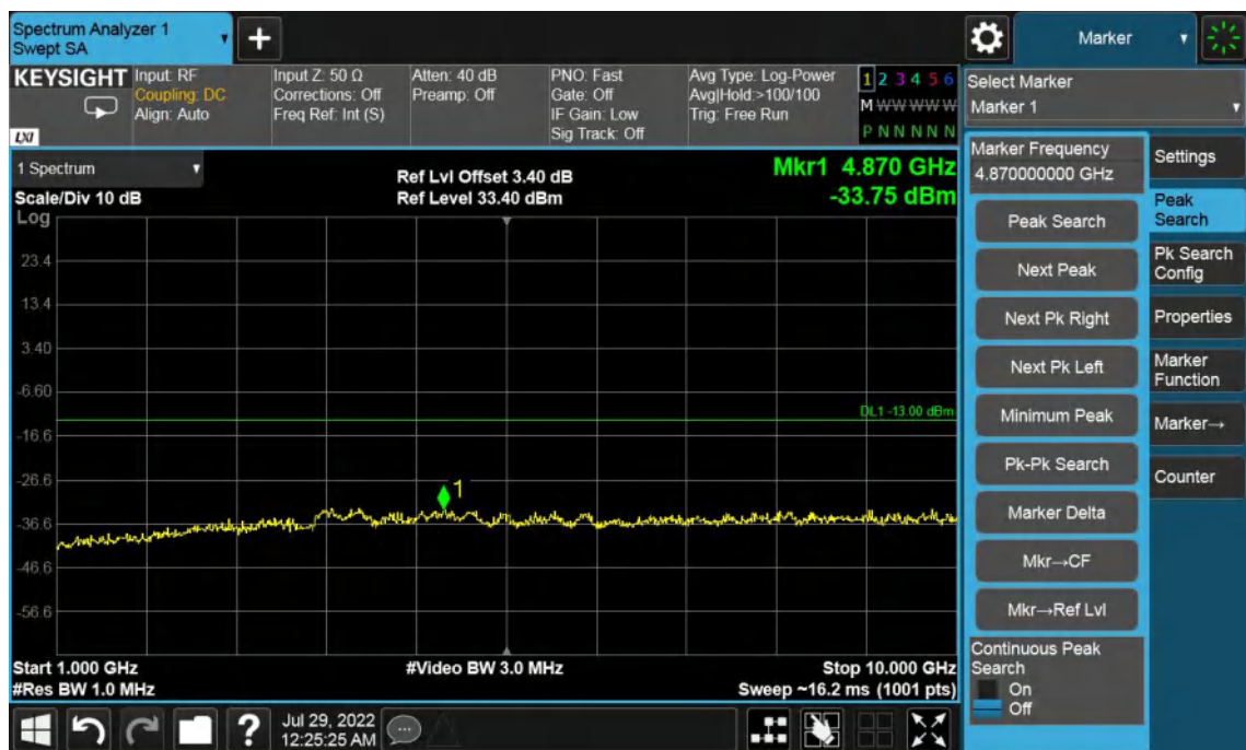
Middle Channel-1.4MHz Bandwidth-1GHz to 10GHz
