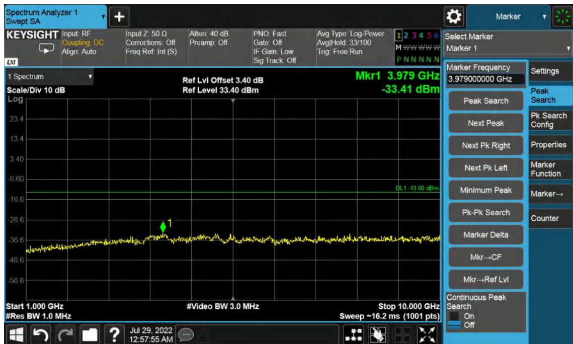
Low Channel-3MHz Bandwidth-1GHz to 10GHz
