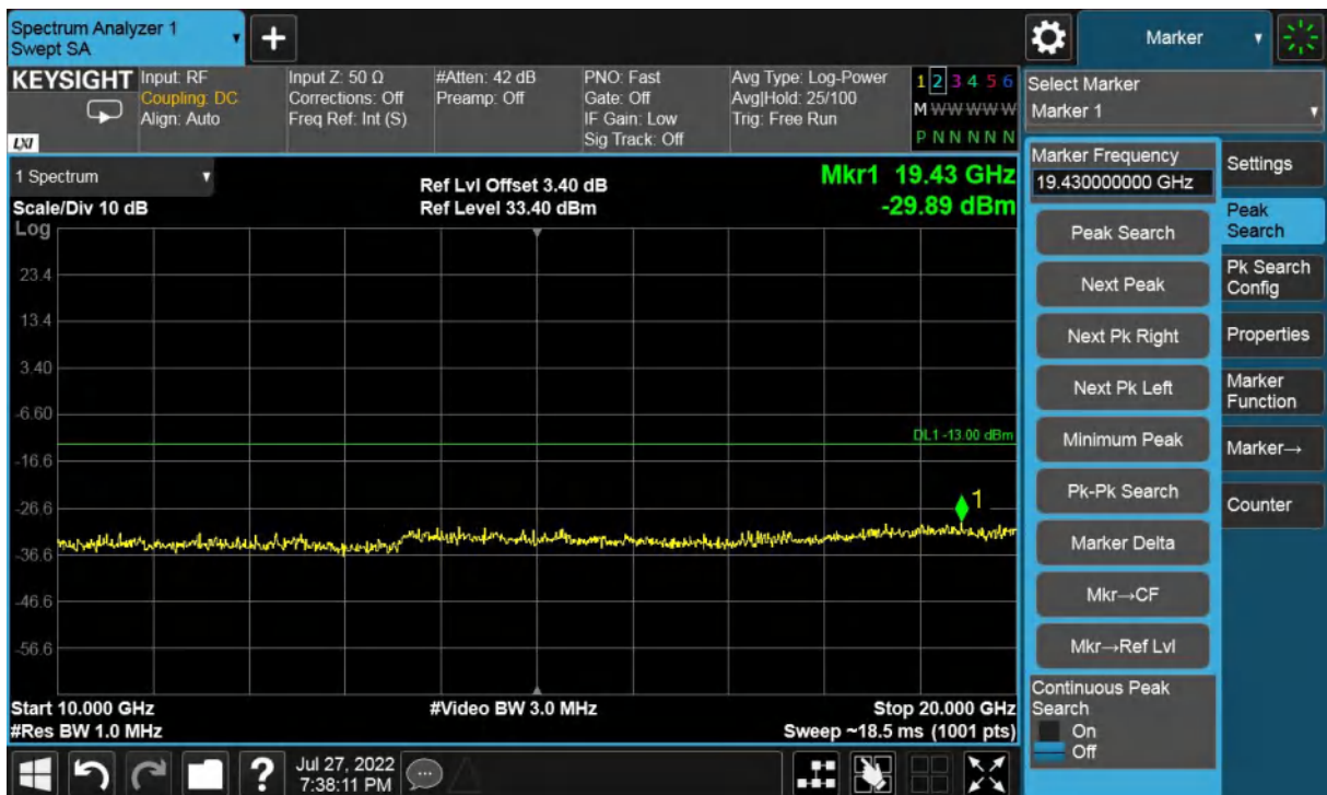
Middle Channel-3MHz Bandwidth-10GHz to 20GHz
