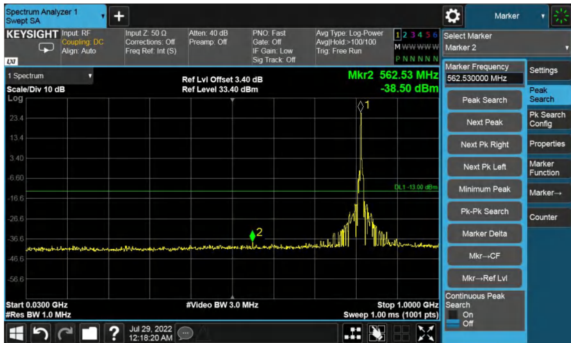
Middle Channel-5MHz Bandwidth-30MHz to 1GHz
