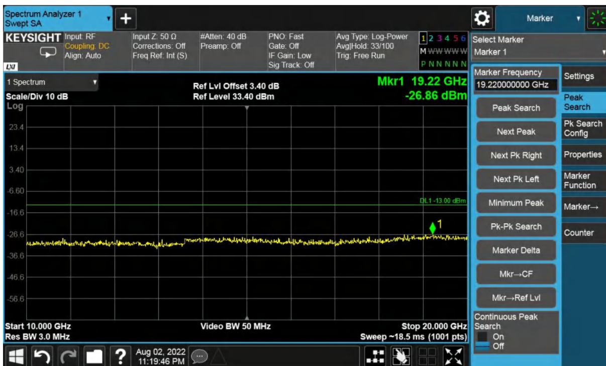
Low Channel-10MHz Bandwidth-10GHz to 20GHz
