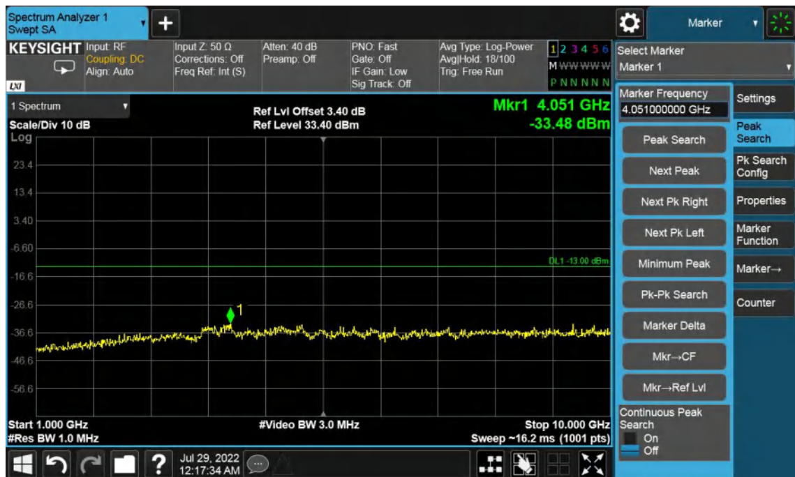
Middle Channel-5MHz Bandwidth-1GHz to 10GHz
