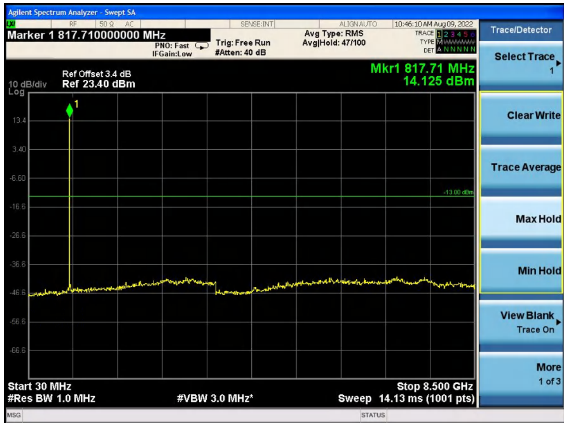
Low Channel-3MHz Bandwidth-30MHz to 1GHz
