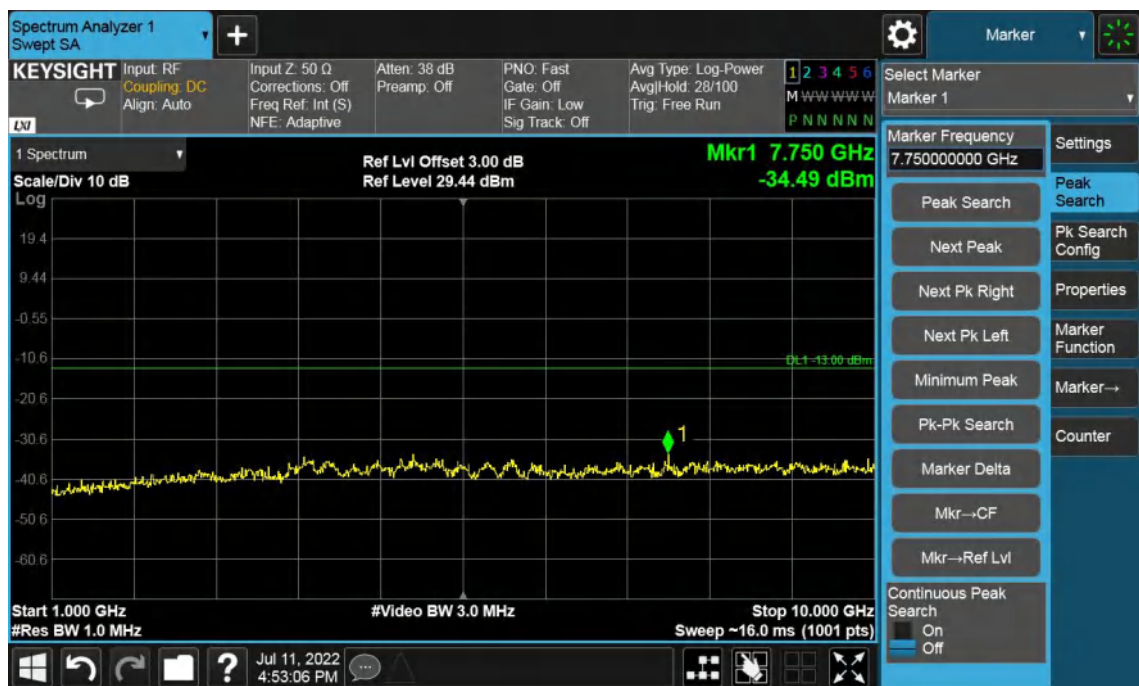
Low Channel-10MHz Bandwidth-1GHz to 10GHz
