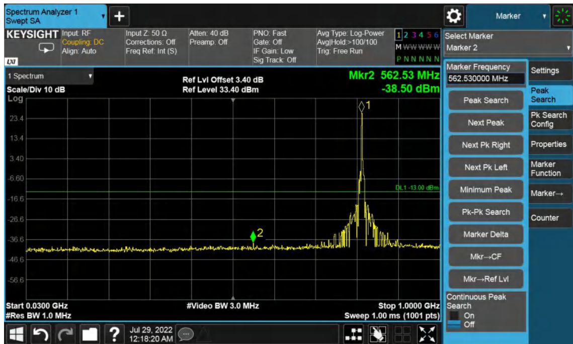
Middle Channel-5MHz Bandwidth-30MHz to 1GHz
