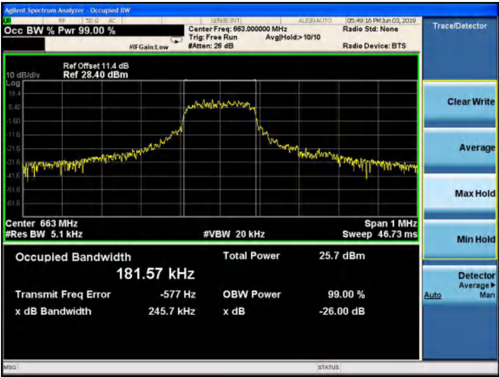
NB-IoT standalone band 71 133122 QPSK(99%)
