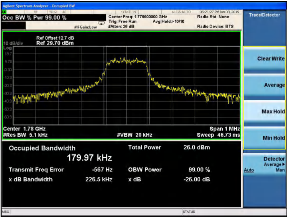
NB-IoT standalone band 66 132671 QPSK(99%)
