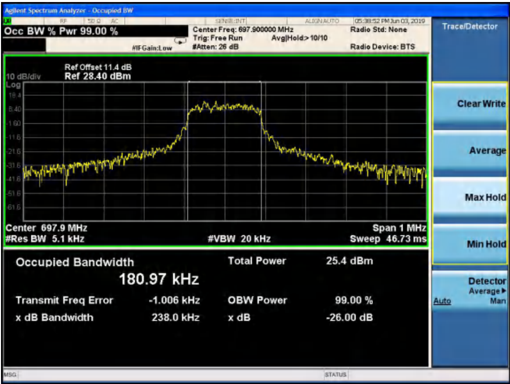
NB-IoT standalone band 71 133471 QPSK(99%)
