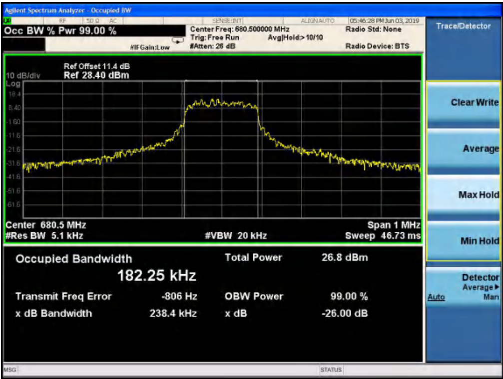
NB-IoT standalone band 71 133297 QPSK(99%)
