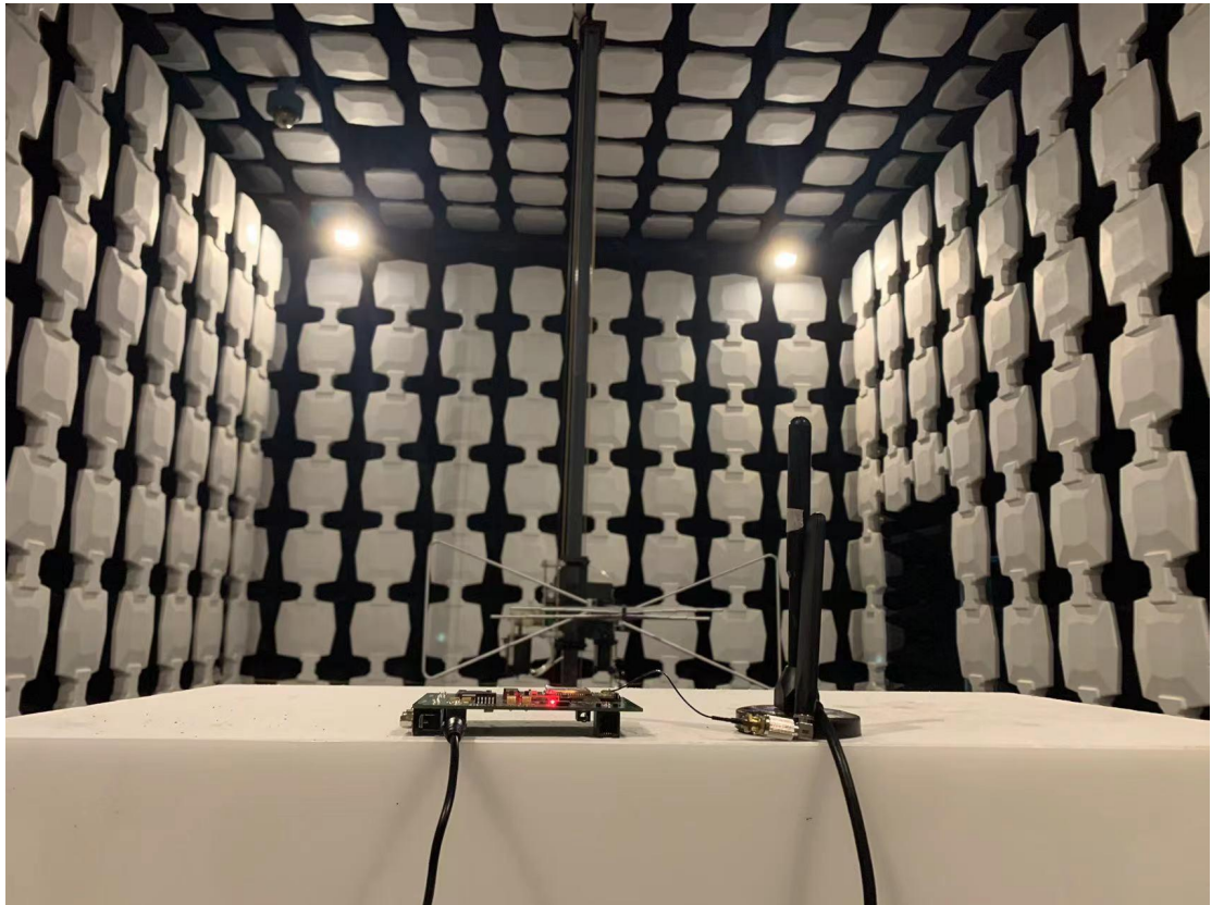
A7672SA miniPCIE RSE 30MHz-3GHz
