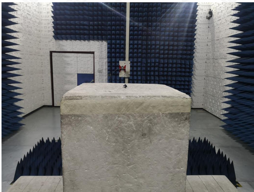
RADIATED EMISSION TEST SETUP ABOVE 1GHZ
