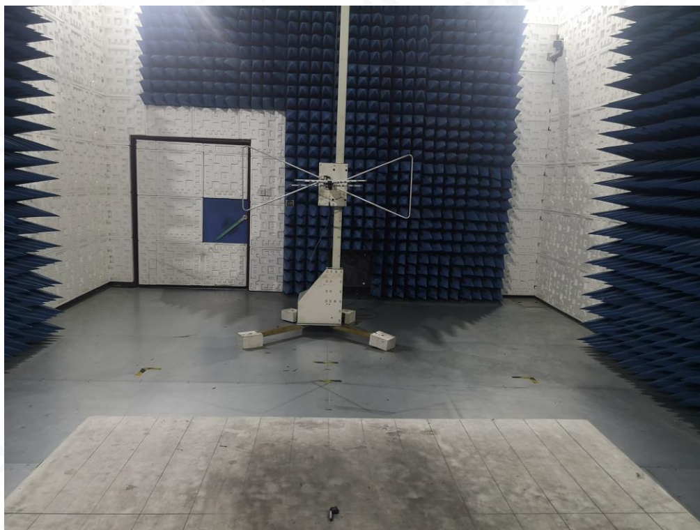
RADIATED EMISSION TEST SETUP ABOVE 1GHZ
