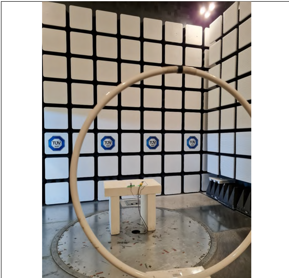
Figure 2 – Radiated Emissions Setup 9kHz to 30MHz
