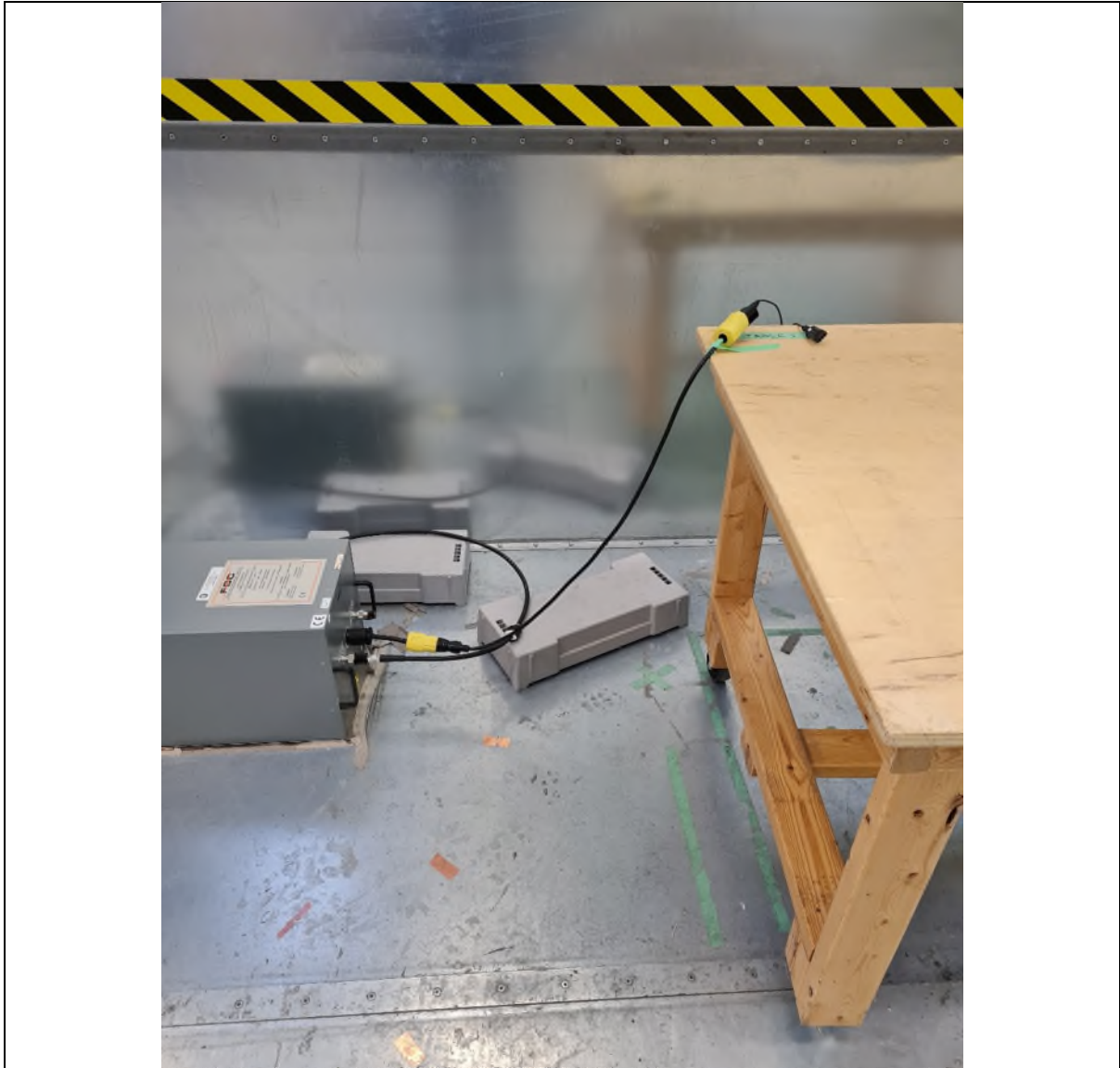
Figure 7 – Power Line Conducted Emissions Setup
