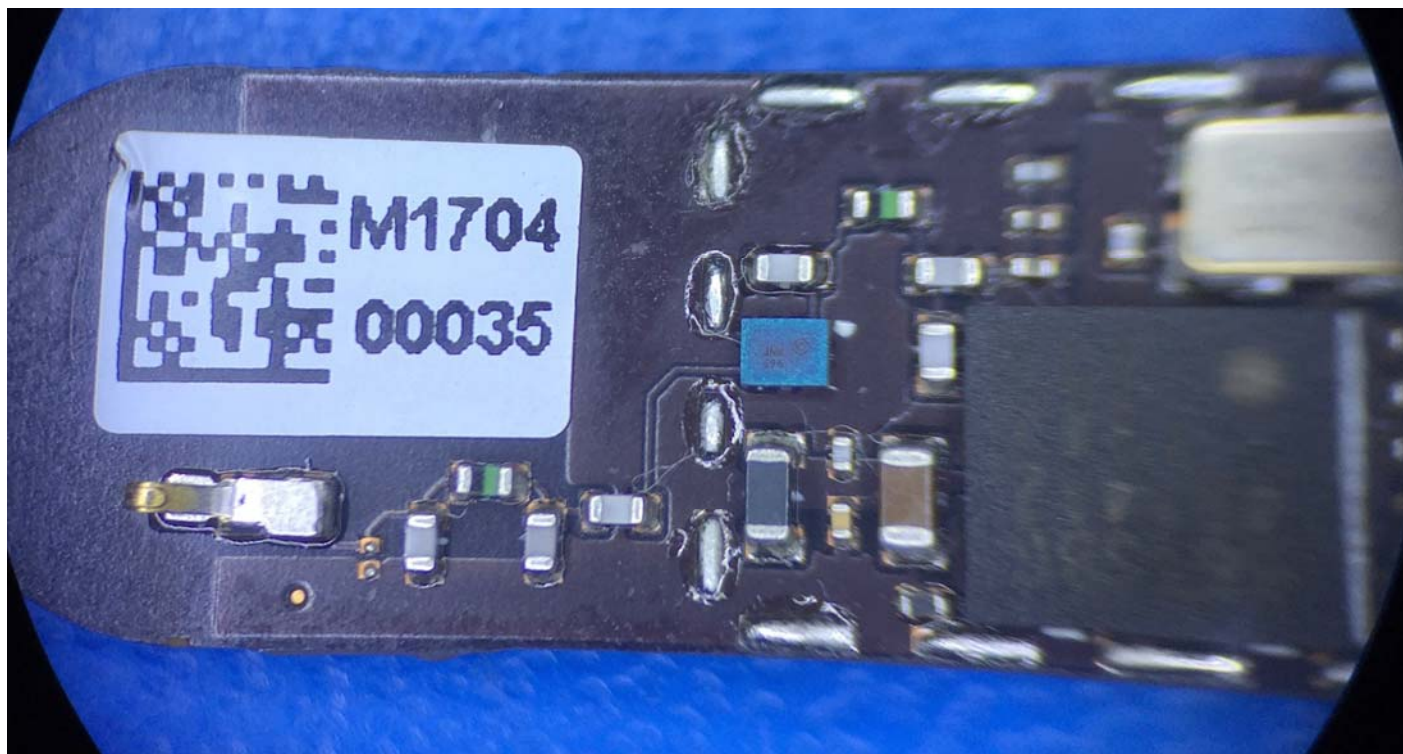
Figure 5 - Beartooth Radio BT 007 - Bluetooth chip & RF section
