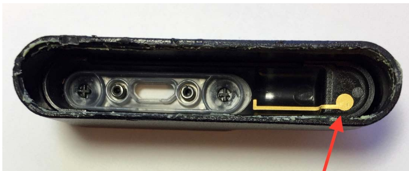
Figure 6 - Beartooth Radio BT 007 - Bluetooth antenna
