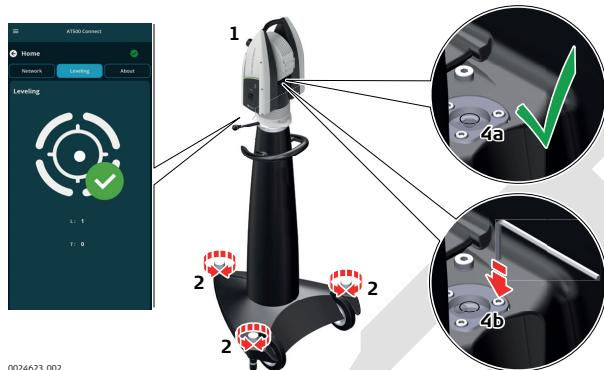
1. Place and secure the instrument into the Quick Release on the Stand Tube.
