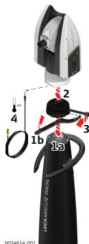
1. Screw the Quick Release onto the Tracker Stand and tighten it using the hinged hook wrench.
