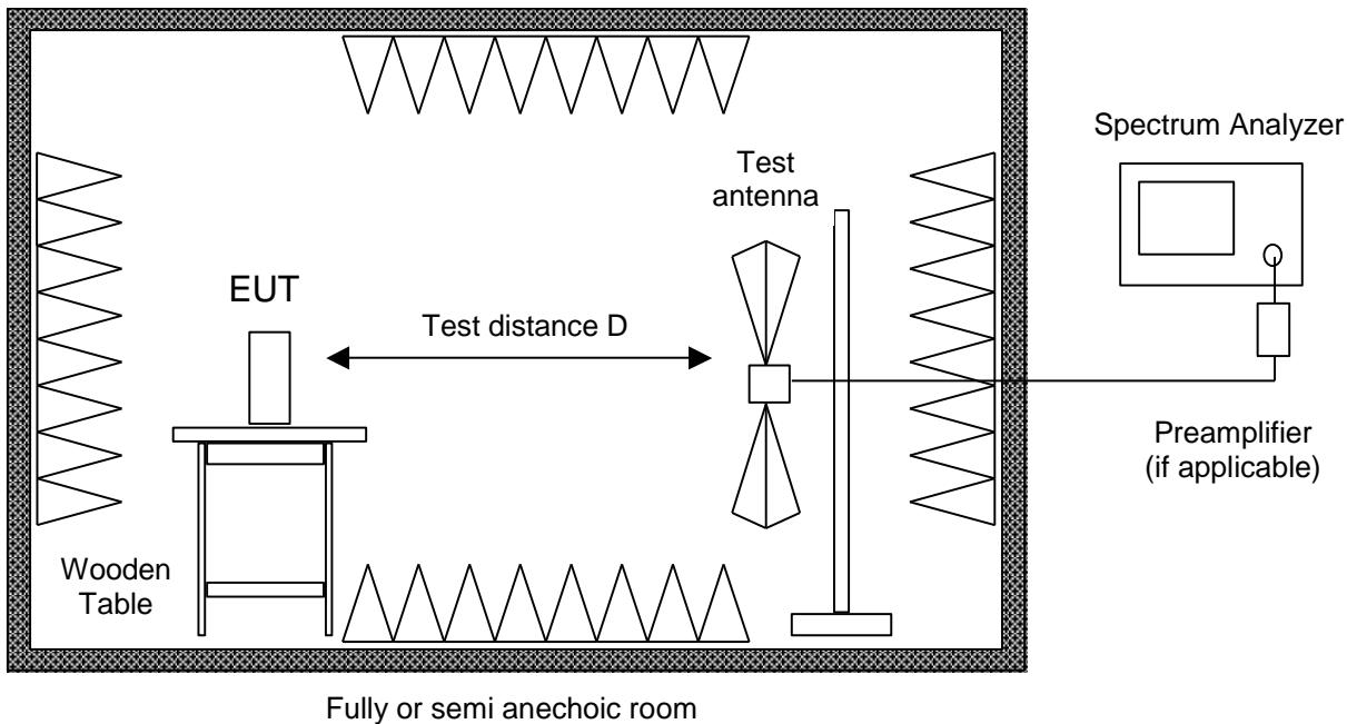
Radiated emission in fully or semi anechoic room is measured in the frequency range from 30 MHz to the maximum frequency as specified in CFR 47 Part 15 section 15.33.
