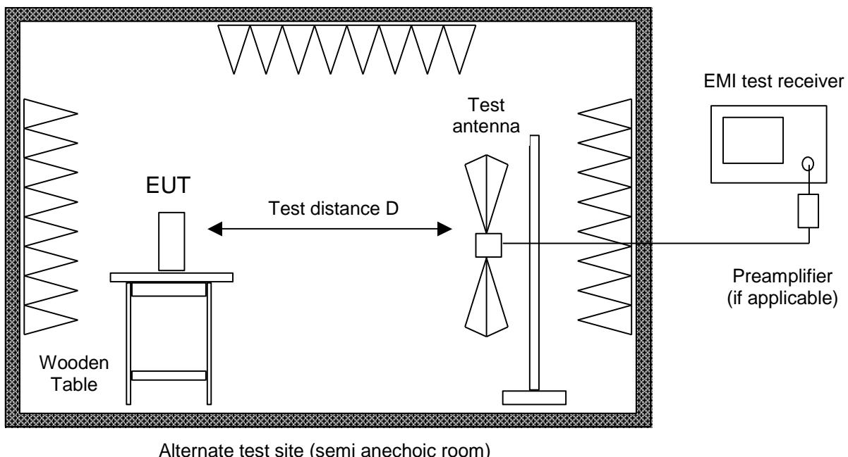
Radiated emission in the frequency range 30 MHz to 1 GHz is measured within a semi-anechoic room with groundplane complying with the NSA requirements of ANSI C63.4 for alternative test sites. A linear polarized logarithmic periodic antenna combined with a 4:1 broadband dipole ("Trilog broadband antenna") is used. The measurement bandwidth of the test receiver is set to 120 kHz with quasi-peak detector selected.
